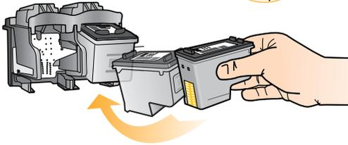
Push both cartridges into carriage until they snap.
