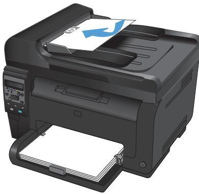
**EN** Test the document feeder and the copy function. Load a printed page into the document feeder face-up. On the control panel, press **Color** or **Black** to start copying.
