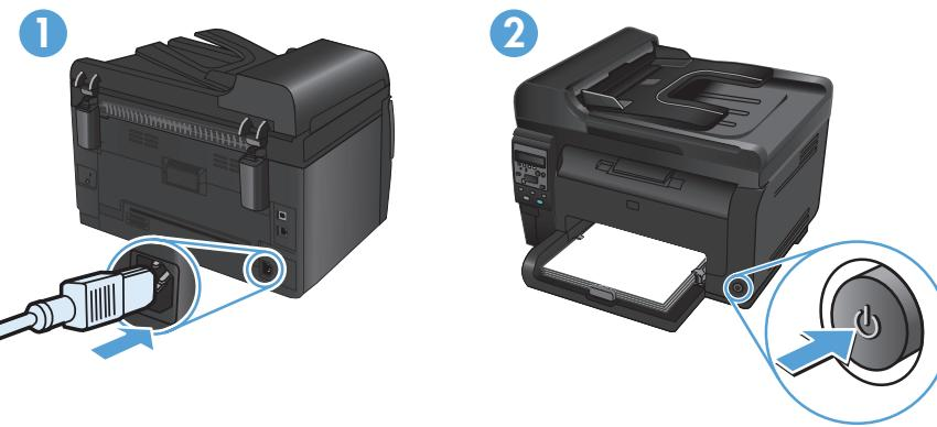
**EN** Connect the power cord between the product and a grounded AC outlet, and then turn on the product. Make sure your power source is adequate for the product voltage rating. The voltage rating is on the product label. The product uses either 110-127 Vac or 220-240 Vac and 50/60 Hz.
