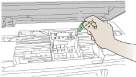
5. Remove the printhead by lifting it straight up.
