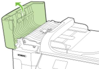
4. Lift the automatic document feeder mechanism.
