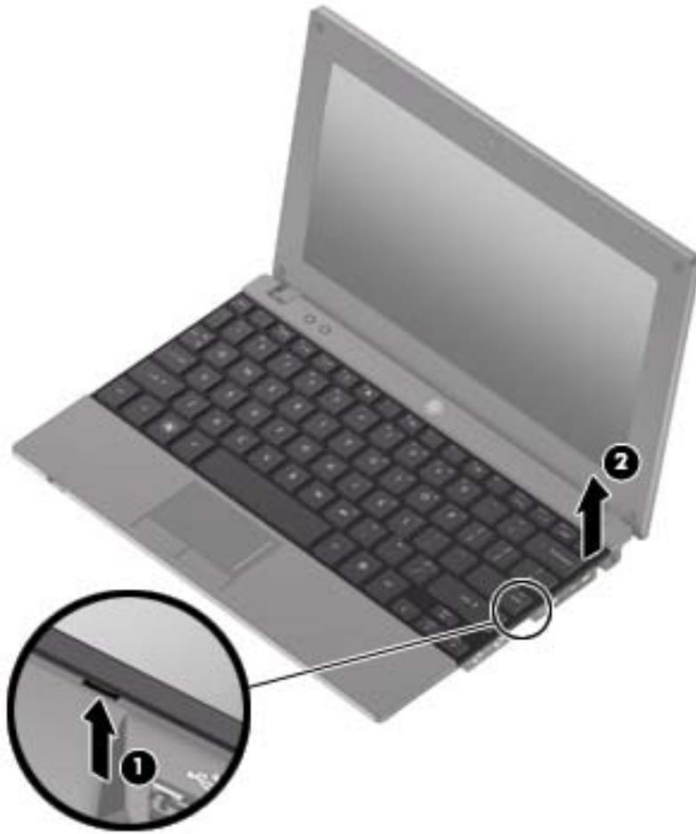
6. Use your right hand to lift up (1) and remove the retention tab from the right side of the top cover (2).
