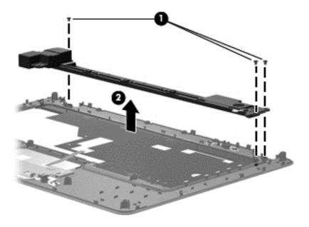
Reverse this procedure to install the speaker assembly.
