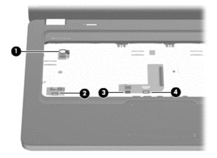
7. Lift the rear edge of the top cover (1) until the top cover disengages from the base enclosure. Remove the top cover (2).
