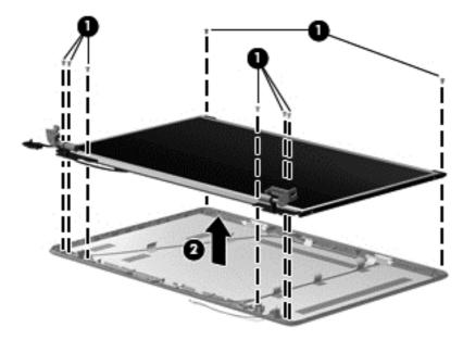
7. Turn the display panel assembly upside down and remove all screws that secure the display panel frame to the display panel.
