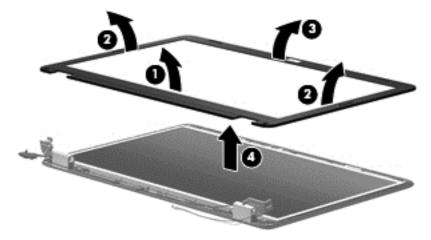
Reverse this procedure to install the display bezel.
