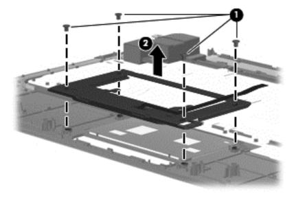
Reverse the above procedure to reassemble and install the TouchPad button board.
