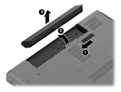
To insert the battery, insert the rear edge of the battery into the battery bay and pivot the front edge downward until the battery is seated. The battery release latch automatically locks the battery into place.
