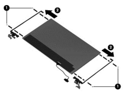
Reverse this procedure to install the display panel brackets.
