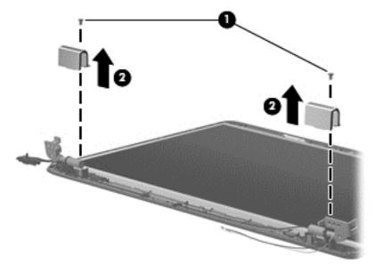
Reverse this procedure to install the display hinge covers.
