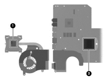
The thermal material must be thoroughly cleaned from the surface of the fan/heat sink assembly (1) and (3), and the processor component (2), each time the fan/heat sink assembly is removed. Thermal pads and thermal paste must be installed on all surfaces before the fan/heat sink assembly is reinstalled.
