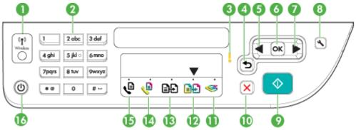
The following diagram and related table provide a quick reference to the device control panel features.
