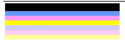
Example of Good Color Bars: All bars are solid, sharp-edged, and extend with uniform color across the entire page. The printer is operating correctly.
