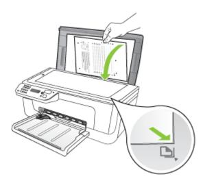
Press OK to scan the alignment sheet.
