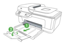
2. Insert the media print-side down along the right of the main tray. Make sure the stack of media aligns with the right and back edges of the tray, and does not exceed the line marking in the tray.
