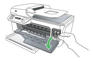
3. Wait until the print carriage is idle and silent, and then lightly press down on the ink cartridge to release it.
