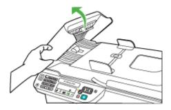
3. Continue lifting the automatic document feeder cover to the vertical position.
