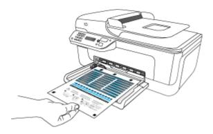
**4.** Place the alignment sheet face down on the scanner glass. For more information, see Load an original on the scanner glass.
