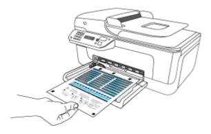
10. Load the ink cartridge alignment sheet face down on the scanner glass in the front right corner with the top of the page to the right, and then press **OK**. For more information, see Load an original on the scanner glass.
