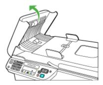
4. Lift the automatic document feeder mechanism.
