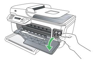
3. Wait until the print carriage is idle and silent, and then lightly press down on an ink cartridge to release it.
