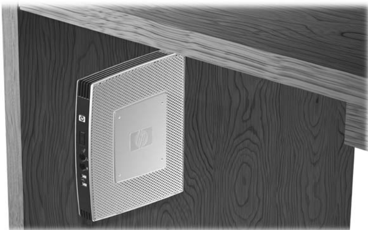
Figure C-8 Thin client mounted under desk
