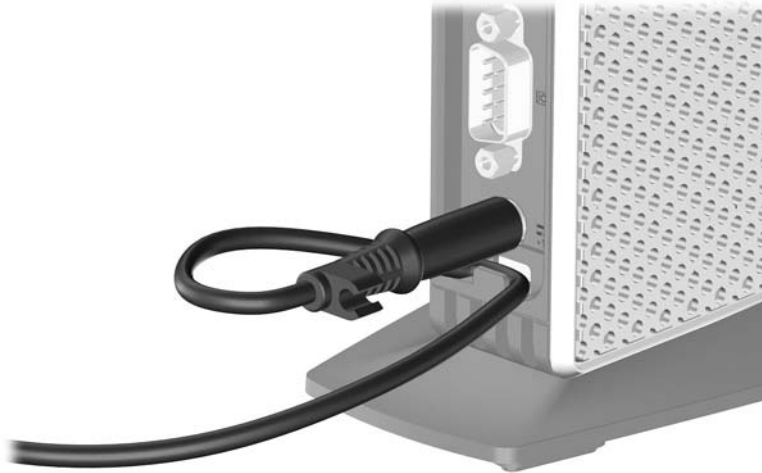
Figure 1-9 Power cord retention slot
