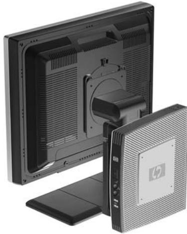
Figure C-6 Thin client mounted on back of monitor stand
