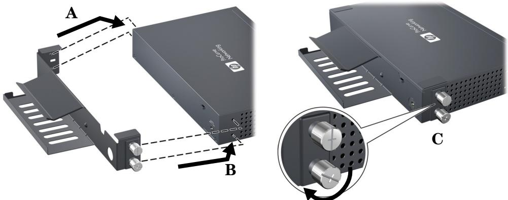
**2.** Insert two alignment pins on one side of the shelf into the appropriate holes on the switch (**A**).
