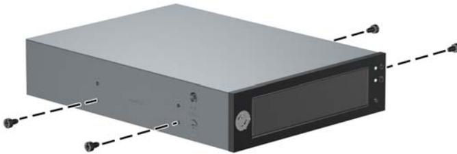
6. Position the guide screws on the drive into the J-slots in the drive bay. Then slide the drive toward the front of the computer until it locks into place.
