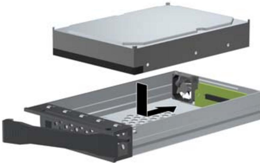
6. Replace the cover by aligning the tab on the rear of the cover with the slot on the rear of the carrier (1) and then rotating the front of the cover onto the carrier (2).
