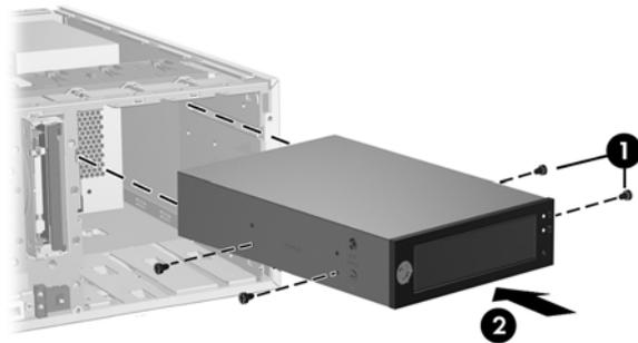
5. Install one (supplied) M3 x 5mm screw (black) for each DX115 unit for shipping support as shown. Additional M3 x 5mm screws are located on the chassis front side under the bezel.
