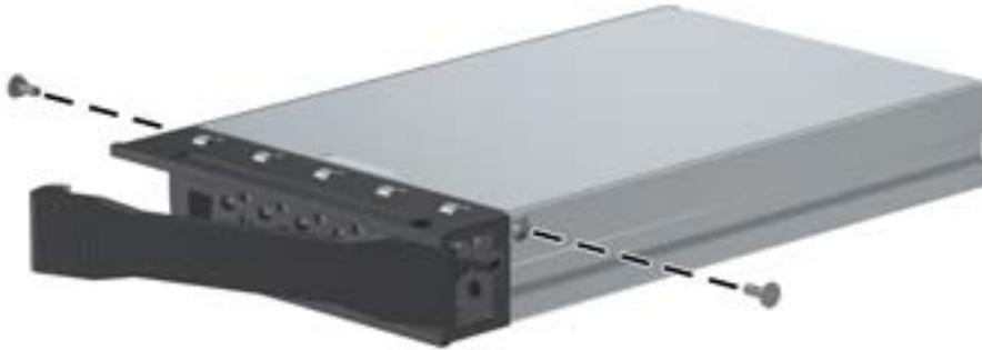
2. Remove the carrier cover by raising the front end of the cover (1) and pulling it away from the slot in the rear of the carrier (2).
