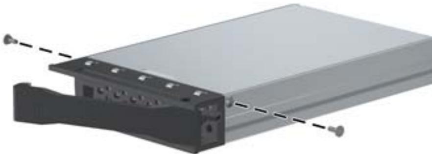
8. With the workstation shut down, insert the carrier into the DX115 unit.
