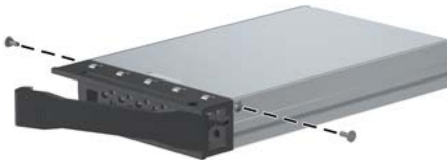
2. Remove the carrier cover by raising the front end of the cover (1) and pulling it away from the slot in the rear of the carrier (2).
