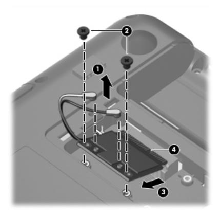
Reverse this procedure to install a WLAN module.
