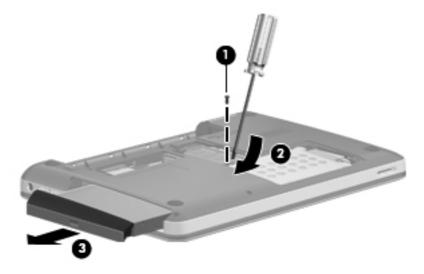
5. If it is necessary to replace the optical drive bracket, position the optical drive with the optical drive bracket toward you.
