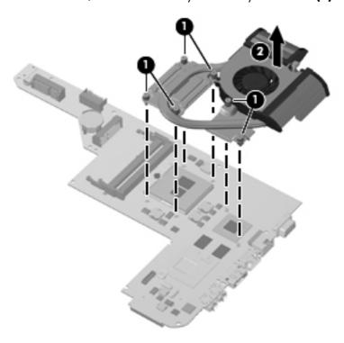
The thermal material must be thoroughly cleaned from the affected surfaces on the system board (1), (3) and from the affected surfaces on the fan/heat sink assembly (2), (4) each time the fan/heat sink assembly is removed. Thermal pads and thermal paste must be installed on all surfaces before the fan/heat sink assembly is reinstalled.
