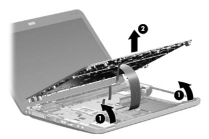
**7.** Release the ZIF connector to which the TouchPad cable is connected and disconnect the cable from the system board **(1)**.
