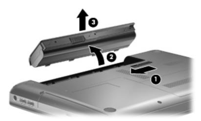
To insert the battery, insert the rear edge of the battery into the battery bay and pivot the front edge downward until the battery is seated. The battery release latch automatically locks the battery into place.
