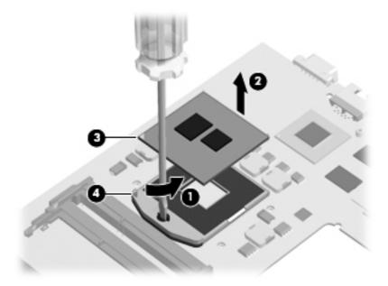
Reverse this procedure to install the processor.
