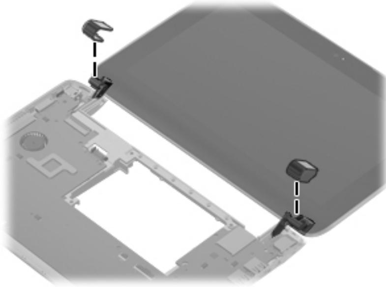
2. Remove the 2 Phillips 2.0x5.0 screws (1) that secure the hinges to the display assembly.
