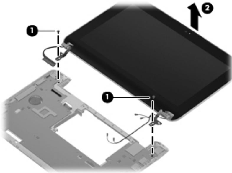
Remove the display assembly hinges:
