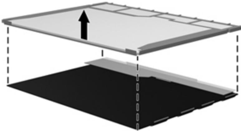
24. Recycle the LCD panel and backlight.
