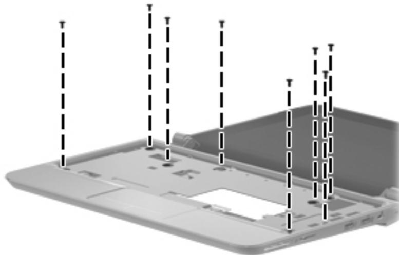
12. Release the top cover by lifting the front edge until it disengages from the base enclosure.
