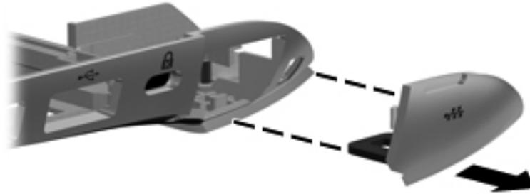
Reverse this procedure to install the RJ-45 cover.
