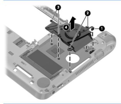
NOTE: The thermal material must be thoroughly cleaned from the surfaces of the fan/heat sink assembly and the system board each time the fan/heat sink assembly is removed: Thermal paste is used on the processor (1) and the fan/heat sink assembly section (2) that services it.
