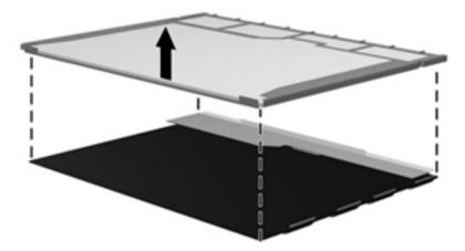
24. Recycle the LCD panel and backlight.
