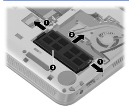
Reverse this procedure to install the memory module.
