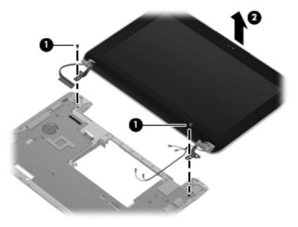
Remove the display assembly hinges:
