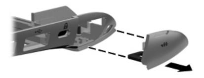
Reverse this procedure to install the RJ-45 cover.
