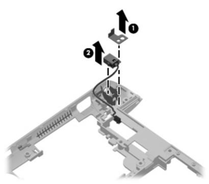
Reverse this procedure to install the power connector cable and DC bracket.
