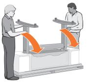
Tilt and lift the printer (1): **WARNING:** 2–3 people for the E+/A0+size model; 2 people for the D/A1-size model. **CAUTION:** Ensure the area in front of the printer is clear of any obstacles such as packaging or rolls of paper.
