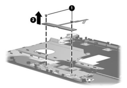
Reverse the above procedure to reassemble and install the TouchPad button board.
