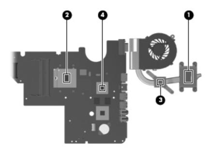
The thermal material must be thoroughly cleaned from the surface of the fan/heat sink assembly (1) and (3), and the processor component (2), each time the fan/heat sink assembly is removed. Thermal pads and thermal paste must be installed on all surfaces before the fan/heat sink assembly is reinstalled.
