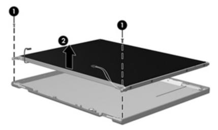
6. Remove the display panel assembly (2) from the display enclosure.
