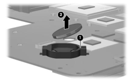
Reverse this procedure to install the RTC battery.
