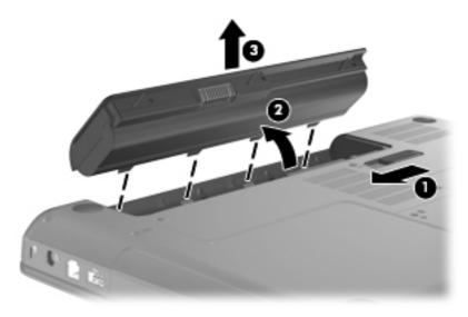
To insert the battery, insert the rear edge of the battery into the battery bay and pivot the front edge downward until the battery is seated. The battery release latch automatically locks the battery into place.
