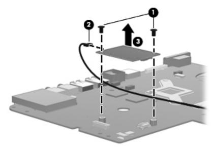
5. Remove the modem module.
