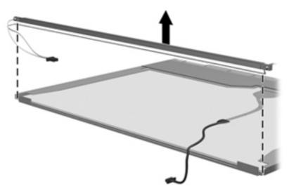
**18.** Remove the backlight from the backlight frame.
