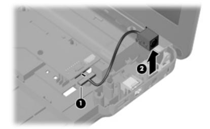
4. Remove the cable from the base enclosure.
