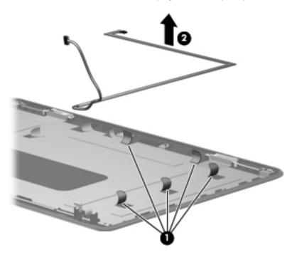
22. If it is necessary to remove the microphone, release the microphone cable from the adhesive strips (1) along the cable path on the display back cover, remove the microphone from the clips on the display back cover (2), and then remove the microphone and microphone cable (3). The microphone and cable is included in the display cable kit, spare part number 592151-001,
