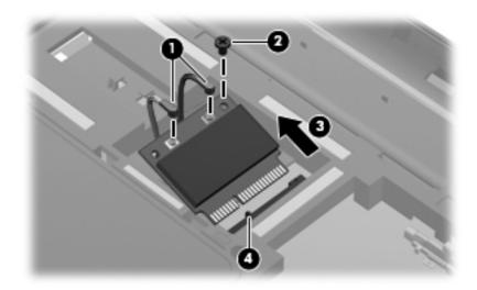
Reverse this procedure to install a WLAN module.
