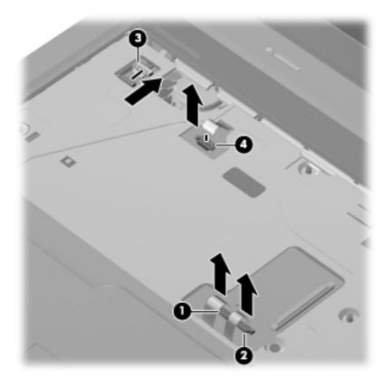
10. Remove the Phillips PM2.5×6.5 screw (1) from the top cover, disengage the rear edge of the top cover (2) from the base enclosure, and then remove the cover from the computer (3).
