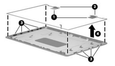
21. If it is necessary to remove the webcam cable, remove the cable from the adhesive strips (1) along the cable path on the display back cover, and then remove the webcam cable (2). The webcam cable is included in the display cable kit, spare part number 592151-001,
