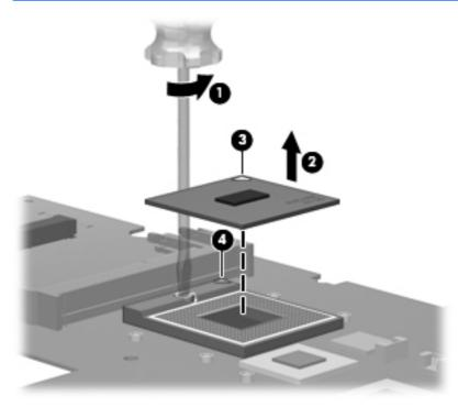
Reverse this procedure to install the processor.
