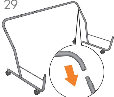
Take the other half of the frame and insert it onto the handle: ensure that the holes are well aligned.
