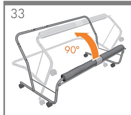
**EN** Rotate the bin structure 90 degrees.
