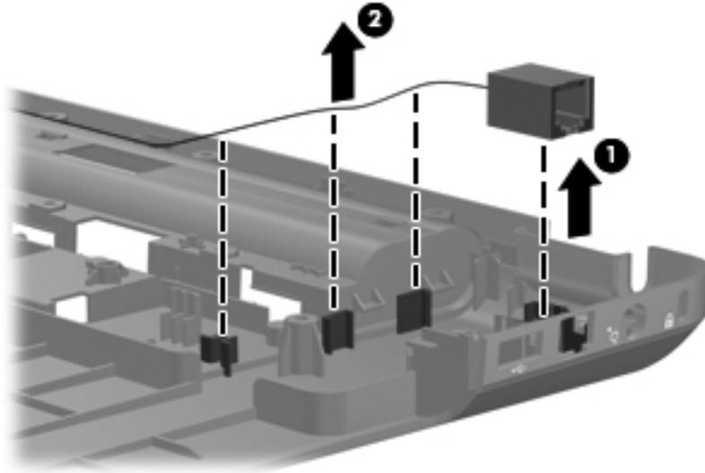
Reverse this procedure to install the RJ-11 connector.
