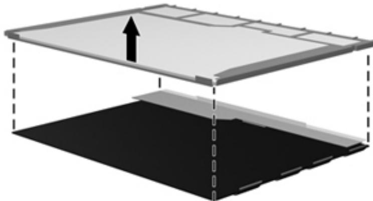
24. Recycle the LCD panel and backlight.
