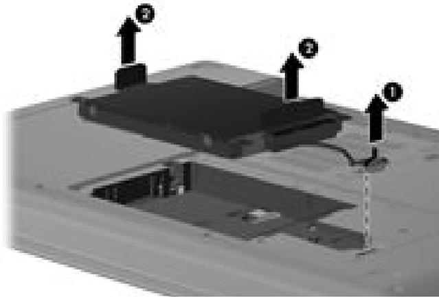
6. If you must remove the hard drive cable, disconnect it from the hard drive.
