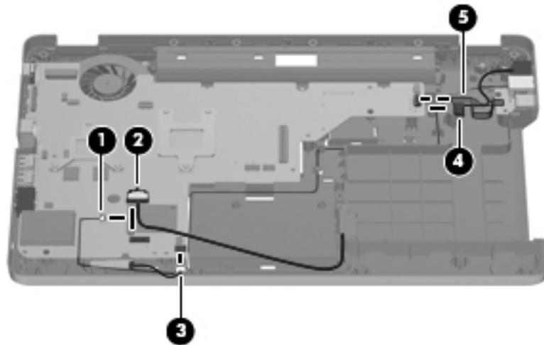
6. Remove the three PM2.5×4.0 screws ❶ that secure the system board to the base enclosure.
