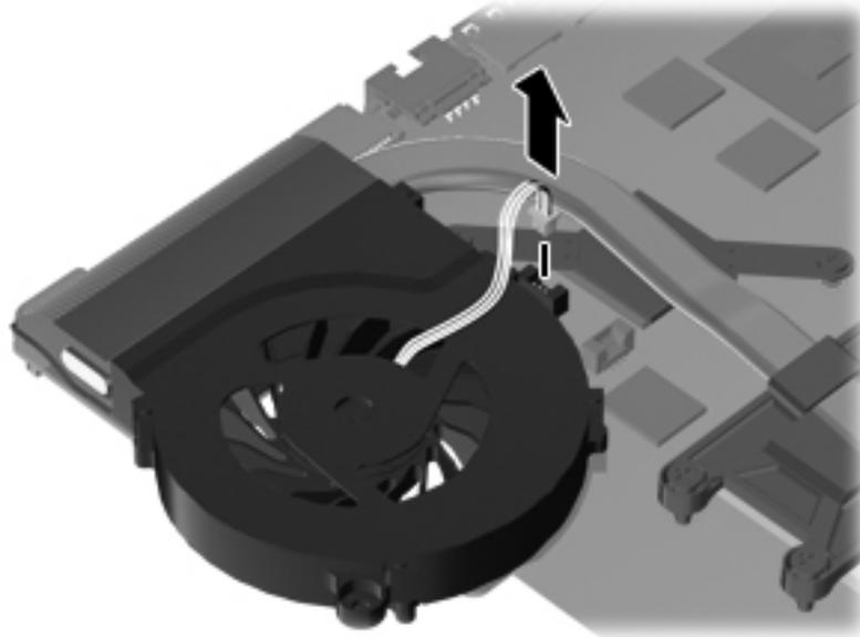
7. Loosen the two Phillips captive screws ① and four Phillips spring-loaded captive screws ② in the sequence shown on the heat sink.
