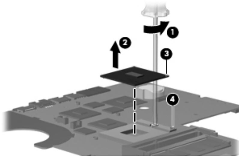
Reverse this procedure to install the processor.
