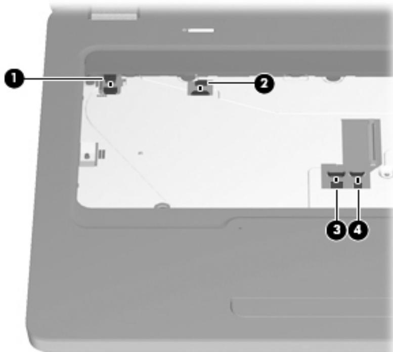
7. Use a small flat-bladed screwdriver to pry along the edges of the top cover to release the top cover ❶ from the base enclosure.
