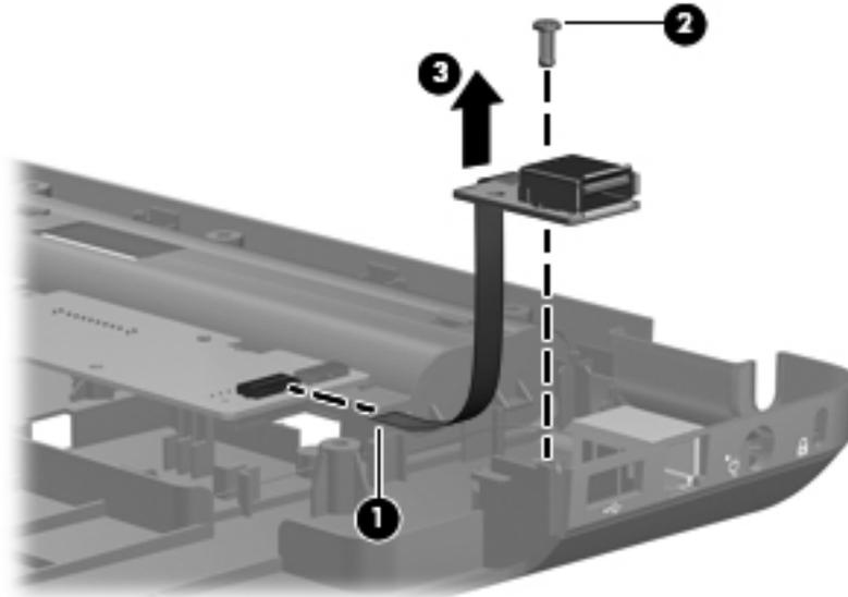
Reverse this procedure to install a USB board.
