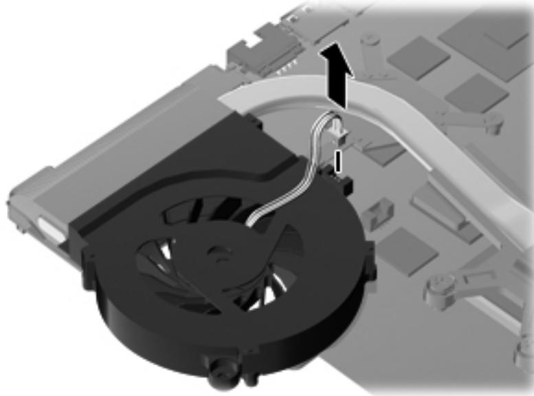
3. Loosen the four Phillips spring-loaded captive screws ❶ that secure the fan/heat sink assembly in the sequence shown on the heat sink.
