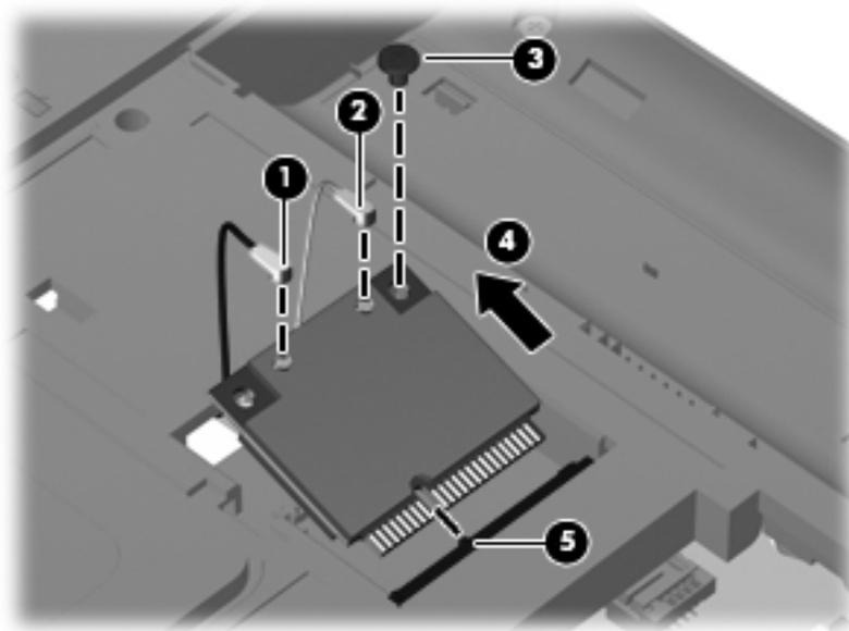
Reverse this procedure to install the wireless module.
