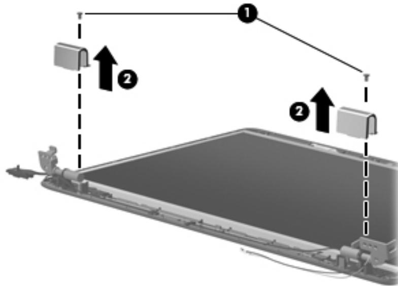
5. Remove all screws ❶ that secure the display panel assembly to the display enclosure.
