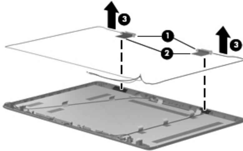
Reverse this procedure to install the display wireless antenna transceivers.
