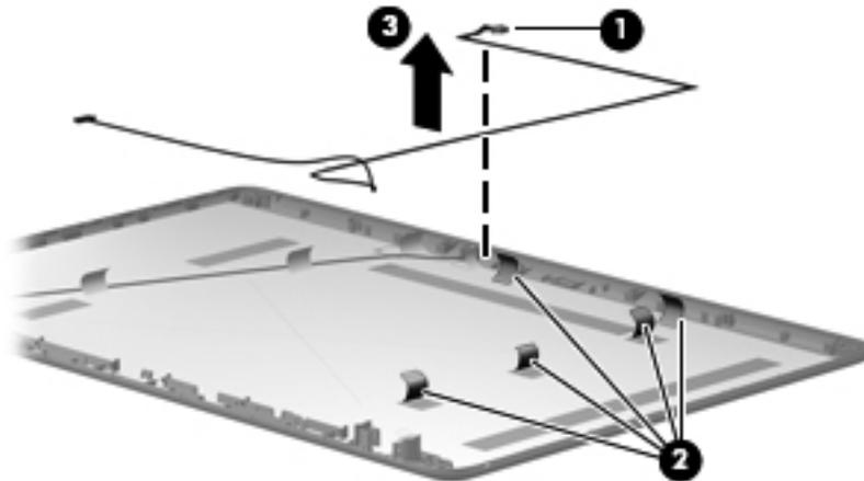
Reverse this procedure to install the webcam cable.
