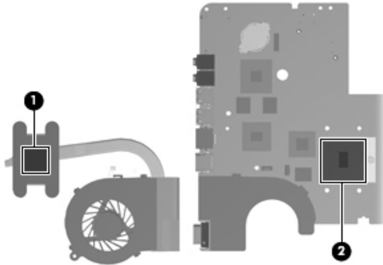
The following illustration shows the replacement thermal material locations for computer models equipped with graphics subsystems with discrete memory.
