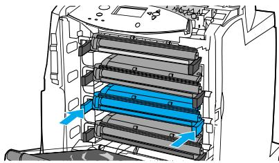
Grasp the blue handles on the sides of the print cartridge. Align the print cartridge with the tracks inside the printer and insert the cartridge until it clicks into place.
