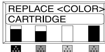
Replace a print cartridge when the printer control panel displays a REPLACE <COLOR> CARTRIDGE message.
