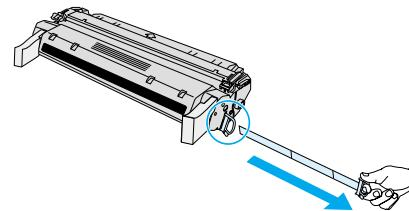
Remove the inside sealing tape by pulling the orange loop on the end of the cartridge and pulling the tape completely out. Discard tape.
