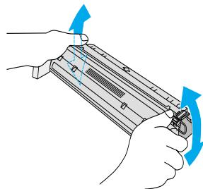
Remove the new cartridge from the bag. Grasp both sides of the cartridge and distribute the toner by gently rocking the cartridge from side to side.
