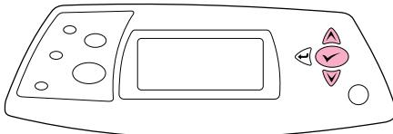
To verify that installation is complete, print a configuration page from the control panel. Press **✓** to open the printer menus. Press **▼** to select INFORMATION, and then press **✓**. Press **▼** to select PRINT CONFIGURATION, and then press **✓**.
