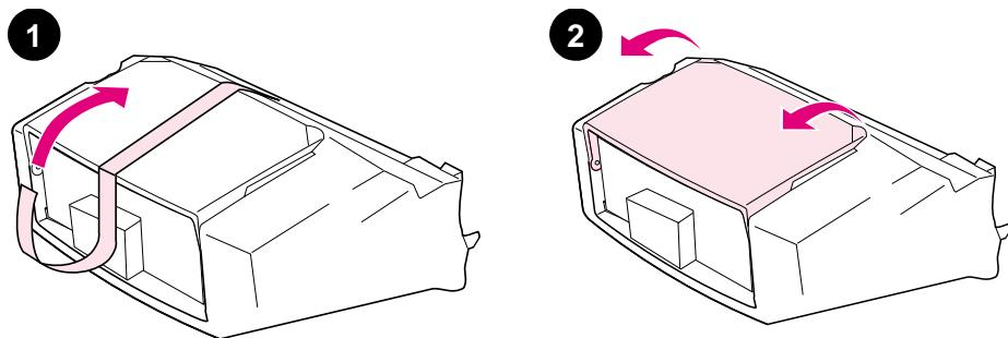
Remove the orange tape from the envelope feeder.
