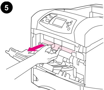
Remove the plastic envelope-entrance cover from inside the printer. **Note:** Replace this cover when the envelope feeder is not attached.
