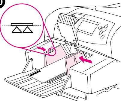
Adjust the guides to touch the envelopes without bending them. **Note:** Make sure that the envelopes are not stacked higher than the arrows on the guides.
