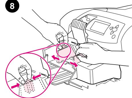
Squeeze the release lever on the left envelope guide and slide the guides apart.
