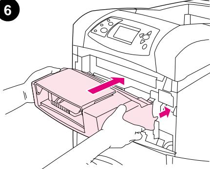
Insert the envelope feeder firmly into the printer until it latches into position. Pull outward on the envelope feeder to make sure that it is securely in place.
