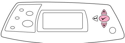
When the envelope-size prompt appears on the control panel display, use the ▲ and ▼ keys to select the correct envelope size, and then press ✓ to save the setting.
