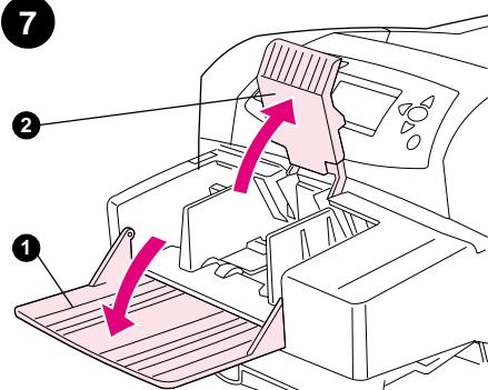
Fold down the envelope-feeder tray (1). Lift the envelope weight (2).
