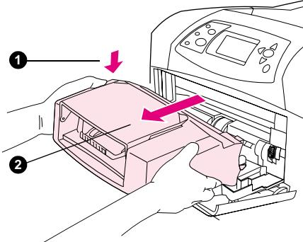
**To remove the envelope feeder.** Press the envelope-feeder release button (1) and pull outward on the envelope feeder (2).
