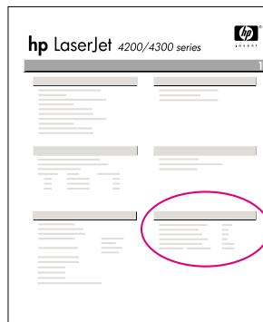
Make sure that the configuration page lists the envelope feeder as an installed accessory. If the feeder is not listed, see the *use* guide on the CD-ROM that came with the printer.
