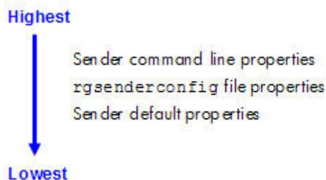
Properties set by methods higher on the list override properties set by methods lower on the list. For example, a Sender command line property can override a property specified in the rgsenderconfig file. Similarly, an rgsenderconfig file property can override a Sender default property.
