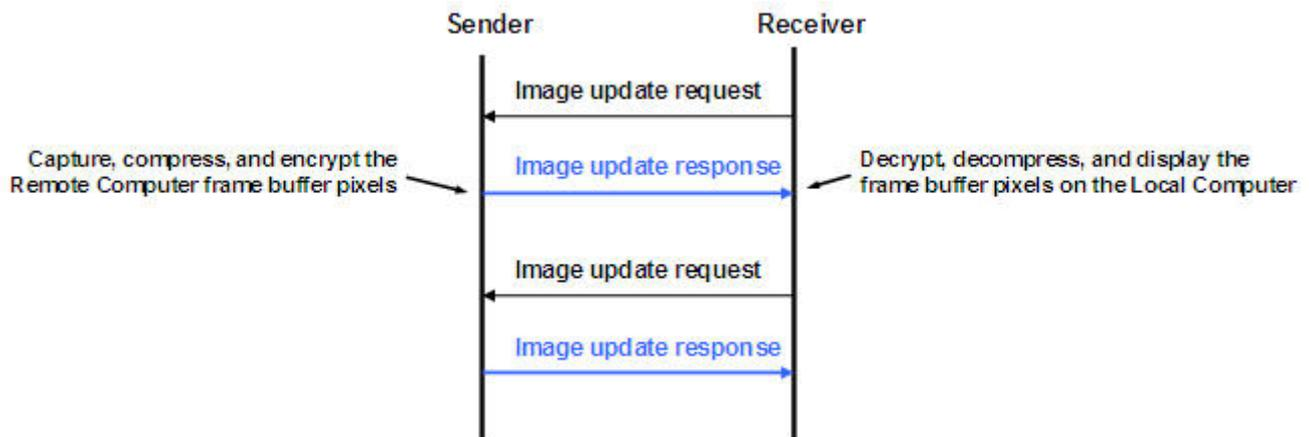
The **Rgreceiver.MaxImageUpdateRequests** property was added to enable performance optimization in high-latency network environments. For example, setting this property to 2 will allow the Receiver to issue a second image update request to the Sender prior to receiving the previous image update response. This allows the Sender and Receiver to operate more in parallel—but at the potential expense of increased network bandwidth consumption.
