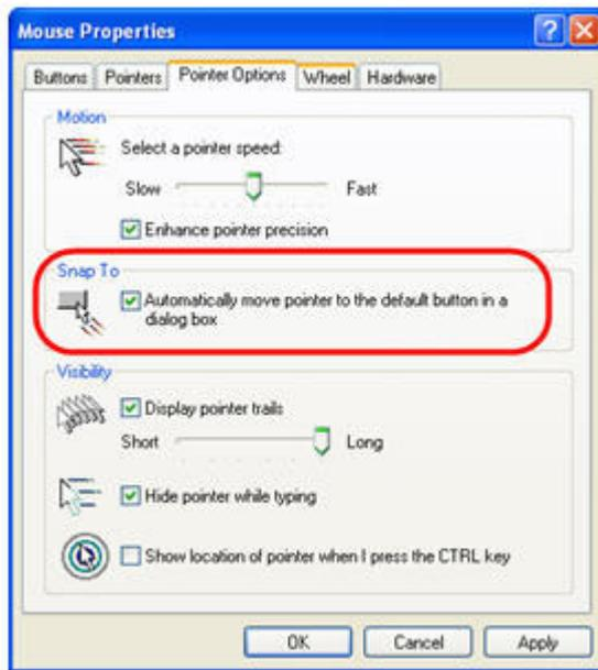
When the `Rgreceiver.IsMouseSyncEnabled` property is set to 1 on the Receiver and when an automatic snap to action occurs on the Sender, the snap to action will be communicated from the Sender to the Receiver; the RGS Receiver will then move the mouse cursor to reflect the cursor position in the Sender dialog box where the snap to action occurred. If this property is set to 0, snap to actions on the Sender will not be reflected on the Receiver.
