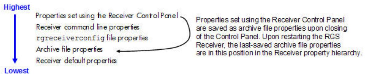
Properties set by methods higher on the list override properties set by methods lower on the list. For example, a Receiver command line property can override a property specified in the `rgreceiverconfig` file. Similarly, an archive file property (saved from the previous Receiver Control Panel session) can override a Receiver default property.
