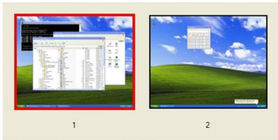
To display the selection dialog, press the **TAB** key while in Setup Mode—again, Setup Mode must have been previously activated by the hotkey sequence. The selection dialog is displayed as long as the initial Setup Mode hotkey (normally the Shift key) remains pressed. The currently-selected Remote Display Window is highlighted with a red border.
