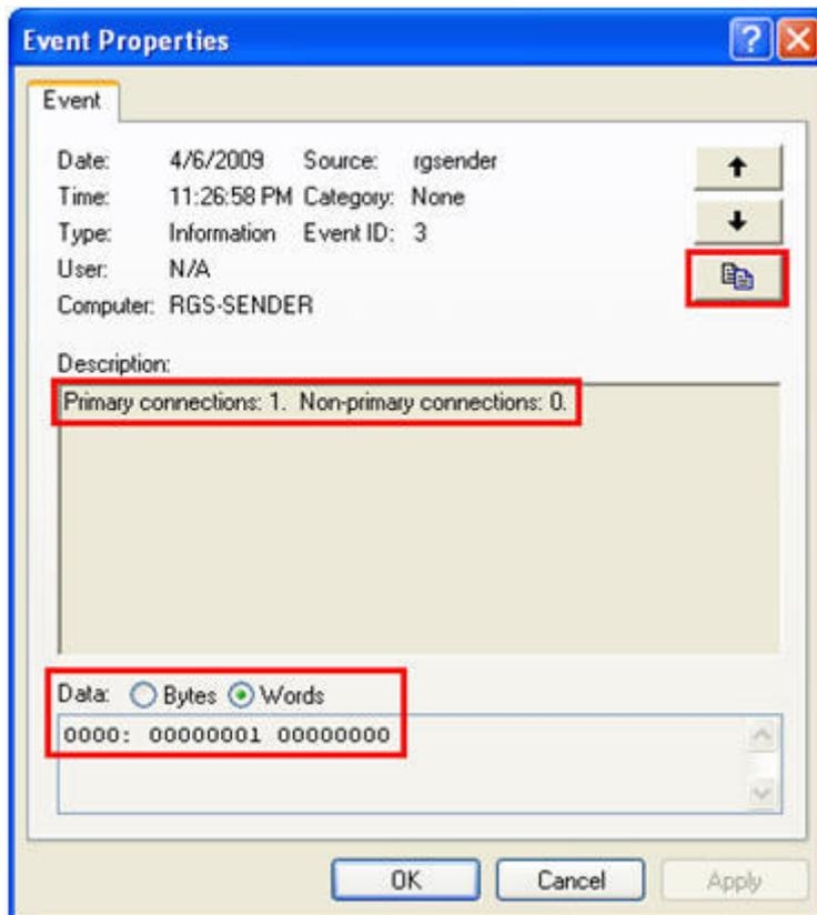
The highlighted radio buttons allow viewing of the connection data (in this case, the number of primary and non-primary connections) in byte and word formats. The Section [HPRemote log format on page 191](#) provides more details on the supported data formats. To copy the details of an event to the Clipboard, click the highlighted button in [Figure 9-2 Event Properties window on page 187](#). By doing a paste into, for example, Notepad, you can view a text listing of the event details.
