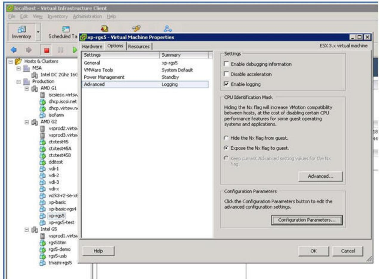
Click the **Configuration Parameters** button in [Figure A-1 Virtual Infrastructure Client GUI on page 216](#) to display the configuration parameters shown in [Figure A-2 Configuration parameters dialog on page 217](#).
