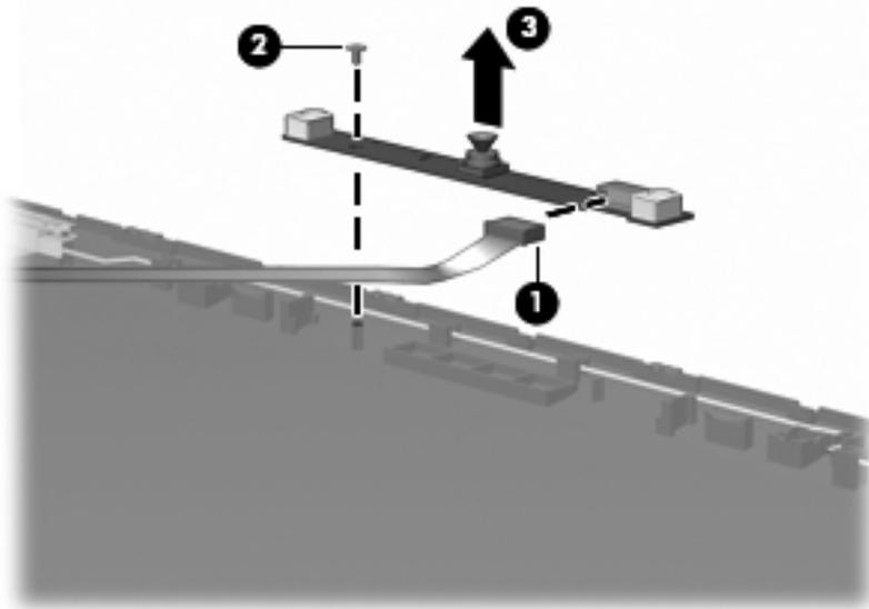
Reverse this procedure to install the webcam/microphone module.
