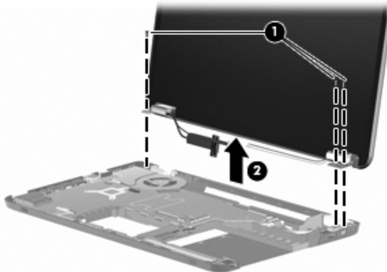
6. To replace the display enclosure or any of the display assembly internal components, remove the following:
