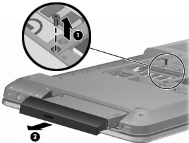
Reverse this procedure to install the optical drive.
