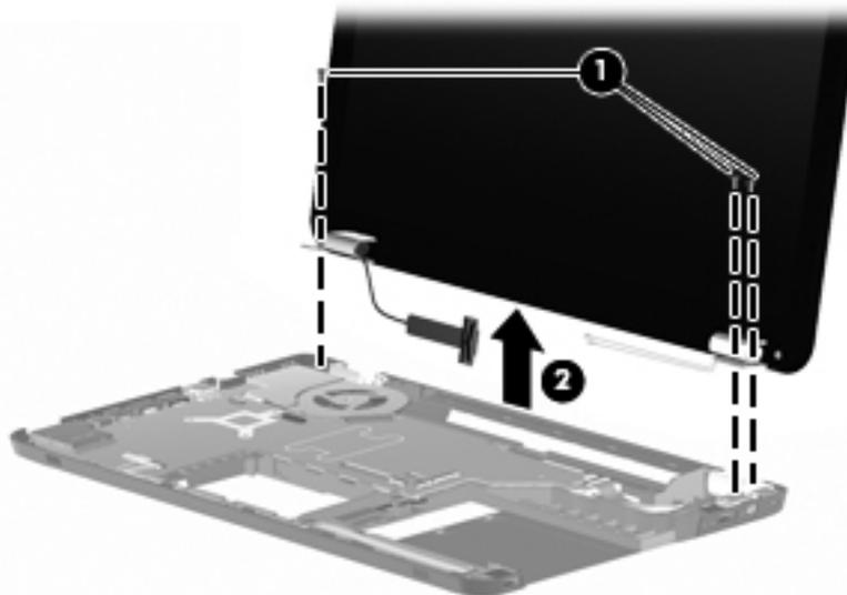
5. To replace the display bezel or any of the display assembly internal components, remove the following:
