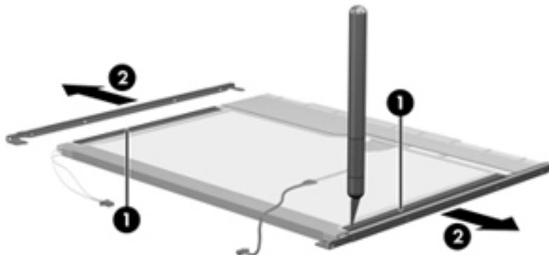
10. Disconnect the display cable (1) from the LCD panel.
