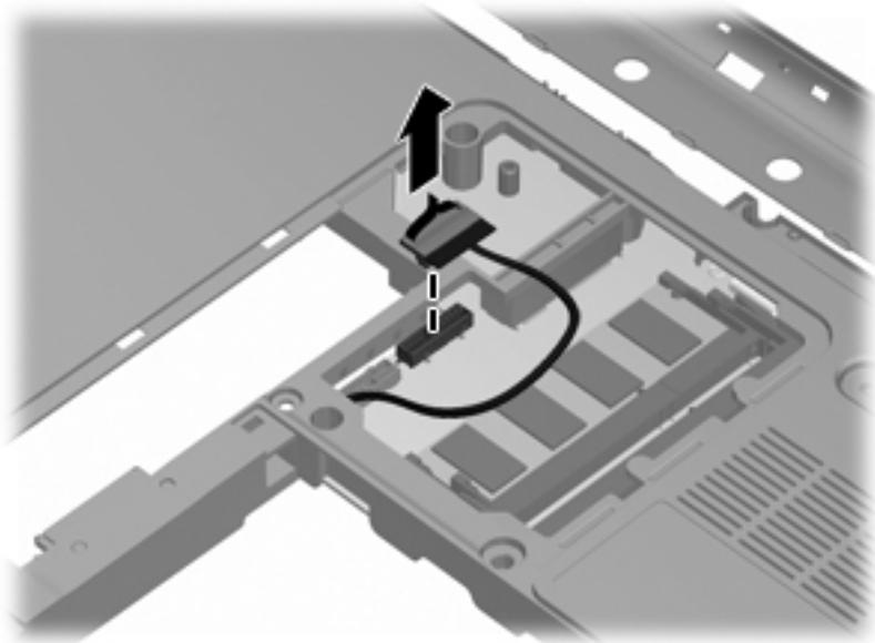
2. Lift up on the right side of the system board until it is at approximately a 45-degree angle (1).
