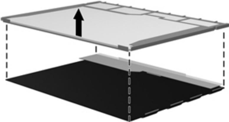
15. Recycle the LCD panel and backlight.
