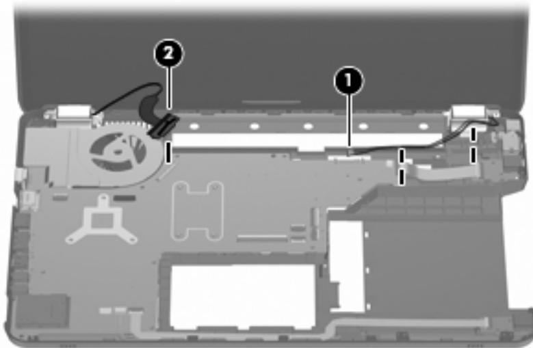
3. Remove the three screws (1) that secure the display assembly to the computer.
