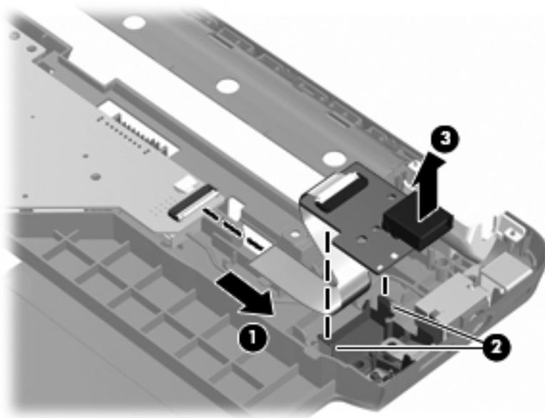
To remove the USB board (left-side):
