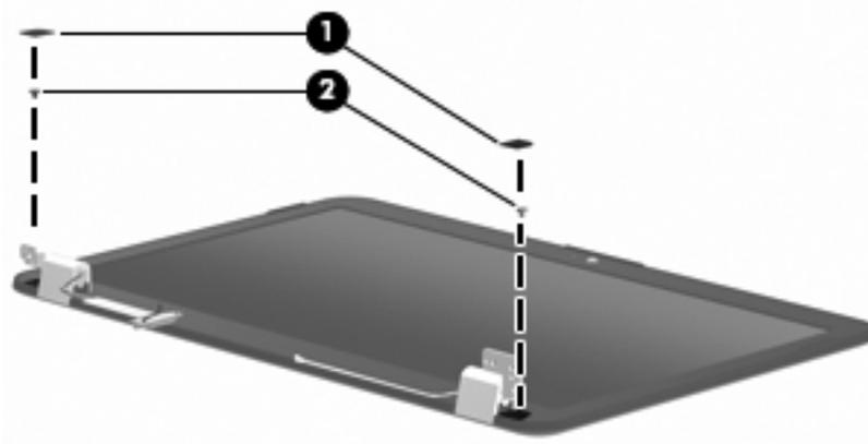
6. Remove the hinge covers by popping off the cover from each hinge.
