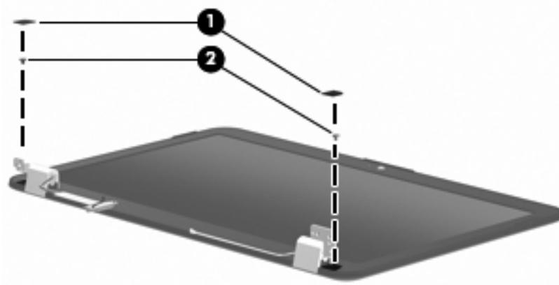
7. To remove the hinge covers, pop off the cover from each hinge.
