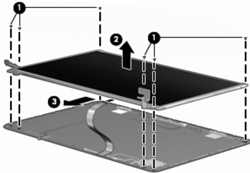
11. To replace the display hinges, remove the three screws (1) that secure each display hinge to the display panel.
