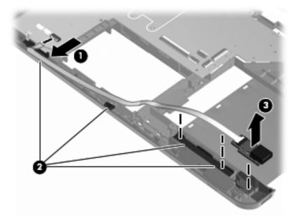
Reverse this procedure to install the front USB board.
