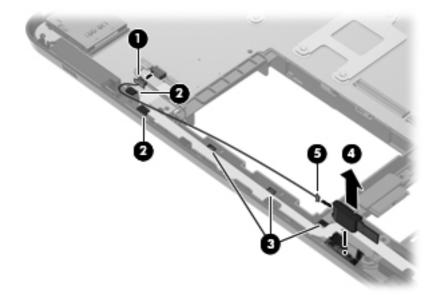
6. Remove the Bluetooth module from the sleeve.
