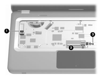
7. Lift the rear edge of the top cover (1) until it rests at an angle.
