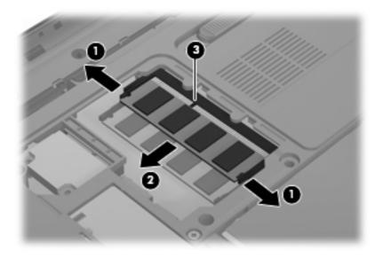
Reverse this procedure to install a memory module.
