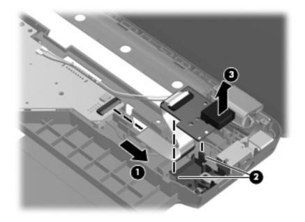
Reverse this procedure to install the rear USB board.
