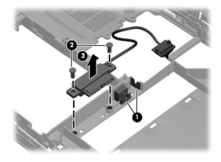
Reverse this procedure to install the optical drive connector board.
