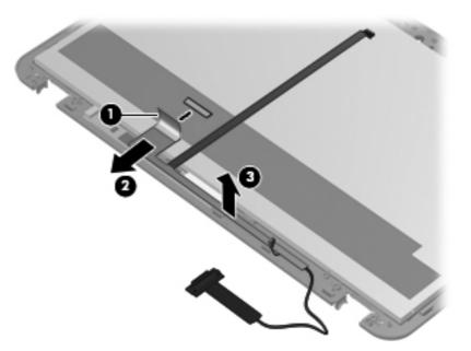
**d.** Remove the display panel cable. The display panel cable is included in the Display Cable Kit, spare part number 603665-001, and includes the webcam/microphone module cable and logo light cable.
