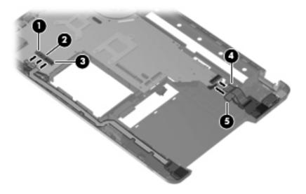
5. Remove the Phillips PM2.5×7.0 screw (1) that secures the display cable channel to the base enclosure.
