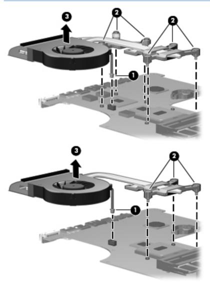
NOTE: The thermal material must be thoroughly cleaned from the surfaces of the fan/heat sink assembly and the system board each time the fan/heat sink assembly is removed. Replacement thermal material locations vary by computer model.
