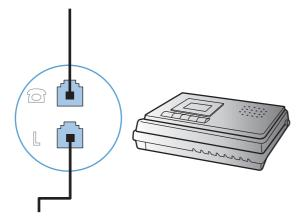
To connect a telephone, plug a telephone cord into the previous device's "telephone" port. Plug the other end of the telephone cord into the telephone "line" port.
