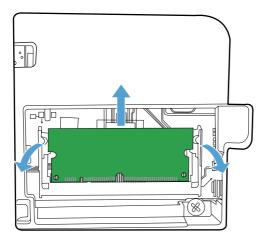
5. Remove the new DIMM from the antistatic package, and then locate the alignment notch on the bottom edge of the DIMM.
