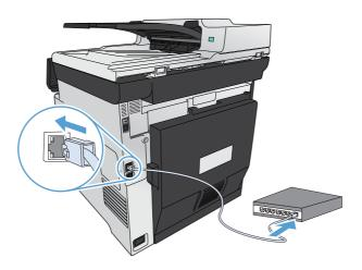
2. Wait for 60 seconds before continuing. During this time, the network recognizes the product and assigns an IP address or host name for the product.
