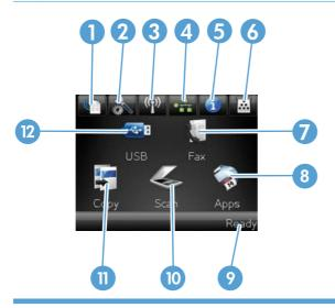
1 Web Services button: provides quick access to HP Web Services features, including HP ePrint.
