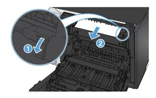
3. If necessary, remove any visible paper from bottom side of the duplexing unit.
