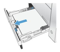
Remove the jammed sheet by pulling it straight out.
