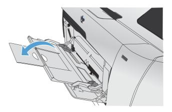
Extend the paper guides fully (callout 1) and then load the paper stack into Tray 1 (callout 2). Adjust the paper guides to the size of the paper.
