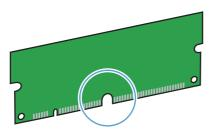
6. Holding the DIMM by the edges, align the notch on the DIMM with the bar in the DIMM slot at an angle.
