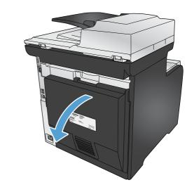
2. If necessary, pull the guide (callout 1) and remove any visible paper (callout 2) from the bottom of the delivery area.
