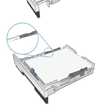
5. Push down on the paper to make sure that the paper stack is below the paper limit tabs on the side of the tray.
