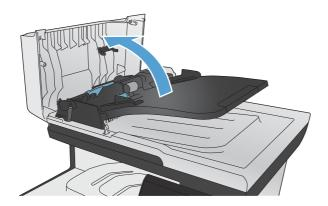
2. Use a moist, lint-free cloth to wipe both pickup rollers and the separation pad to remove dirt.
