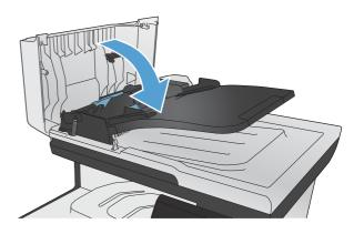
6. Open the scanner lid. If paper is jammed behind the white plastic backing, gently pull it out.
