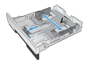
To load Legal-size paper, extend the tray by pressing and holding the extension tab while pulling the front of the tray toward you.
