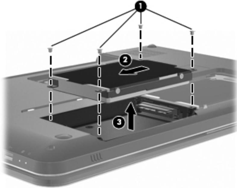
Reverse this procedure to install the secondary hard drive.
