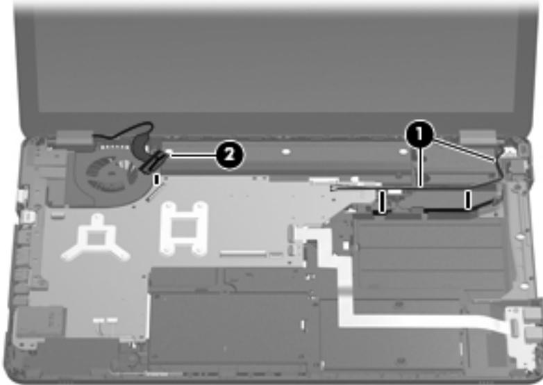
2. Remove the two Phillips PM2.5×5.0 screws **(1)** that secure the display assembly to the computer.
