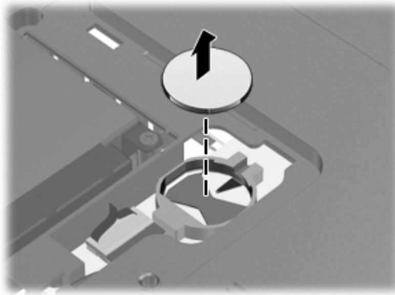
Reverse this procedure to install the RTC battery. Be sure that the RTC battery is installed with the “+” sign facing up.
