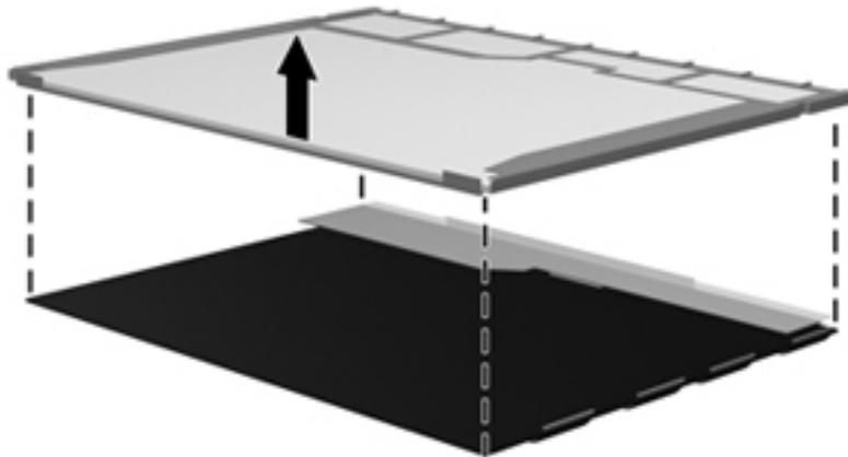
**24.** Recycle the LCD panel and backlight.
