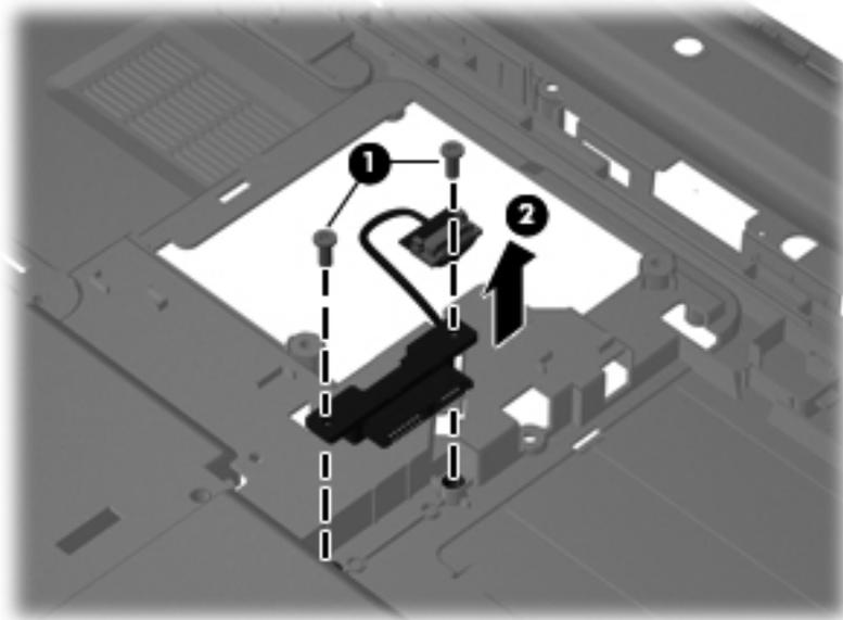
Reverse this procedure to install the optical drive connector.
