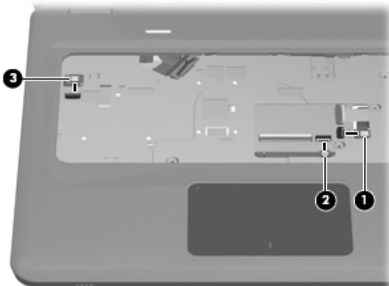
8. Lift the top cover **(1)** and remove from the computer **(2)**.
