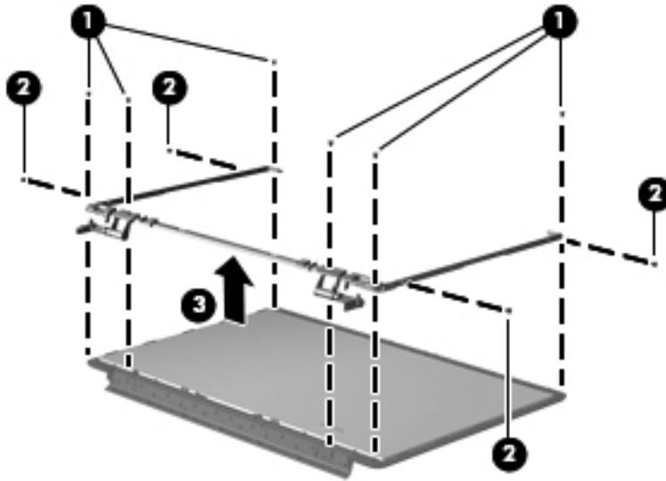
The left and right sides of the display hinge assembly are secured using four PM 2.5×4.0 screws (1) to a bracket (2) as shown in the following image.
