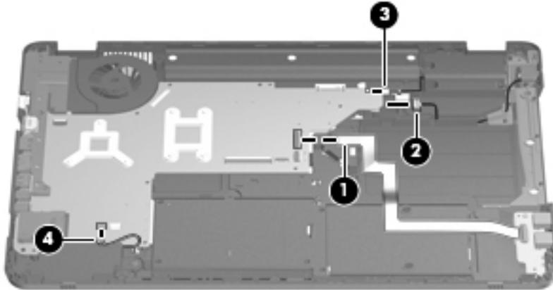
2. Remove the two Phillips PM2.5x5.0 screws (1) that secure the system board to the base enclosure.
