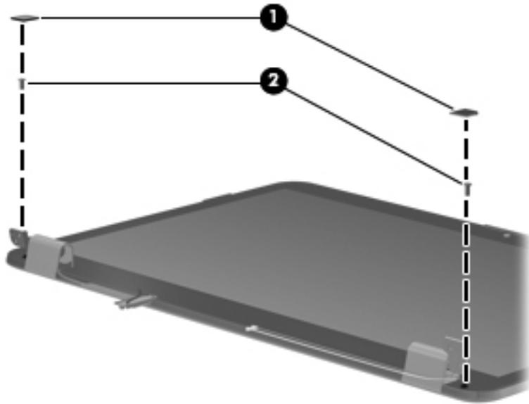
**19.** Slide off each hinge cover to remove from the display assembly.
