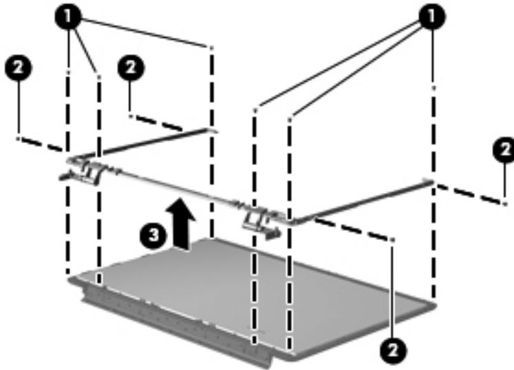
The left and right sides of the display hinge assembly are secured using four PM 2.5×4.0 screws **(1)** to a bracket **(2)** as shown in the following image.
