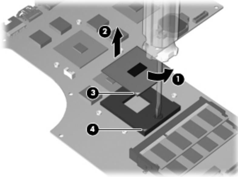
Reverse this procedure to install the processor.
