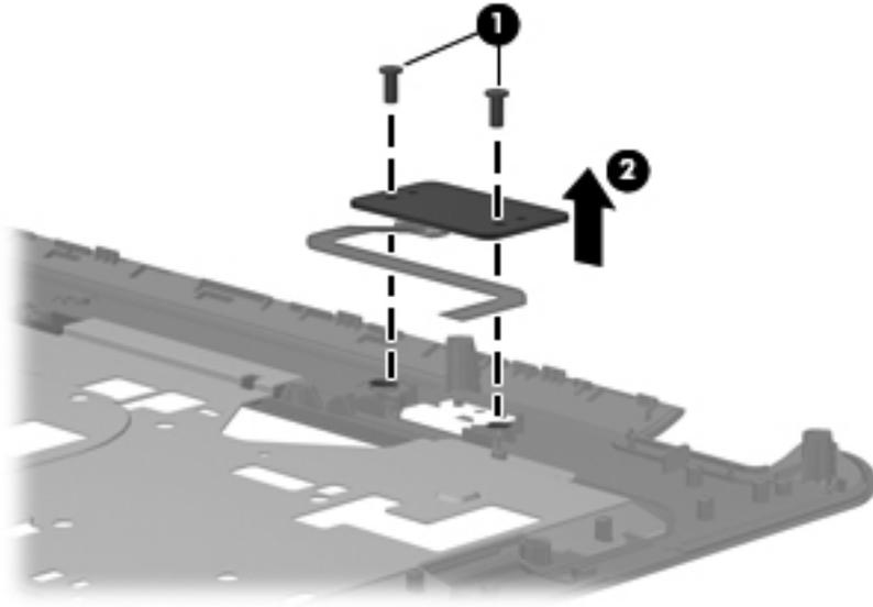
Reverse this procedure to install the power button board.
