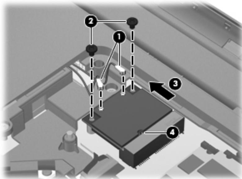
Reverse this procedure to install a WLAN module.
