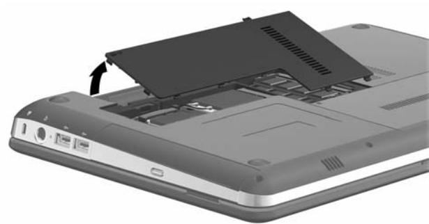
3. Remove the memory module/wireless module compartment cover. The memory module/wireless module compartment cover is included in the Plastics Kit, spare part number 606892-001.
