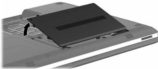
3. Remove the hard drive cover. The hard drive cover is included in the Plastics Kit, spare part number 606892-001.
