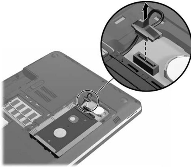
5. Lift the hard drive straight up and remove it from the hard drive bay.
