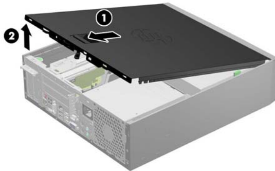
Figure 2-1 Removing the Computer Access Panel
