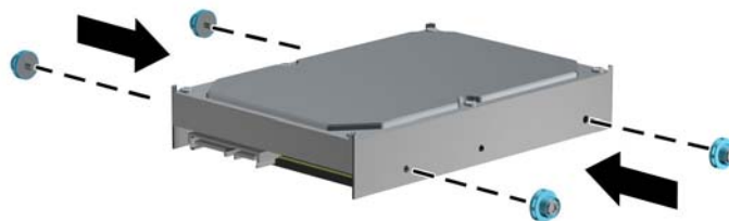
Figure 2-62 Installing Primary Hard Drive Guide Screws
