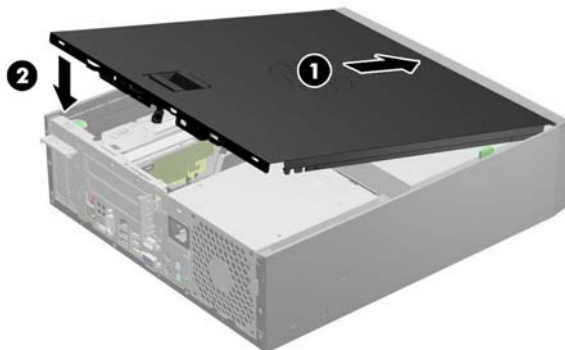
Figure 2-2 Replacing the Computer Access Panel
