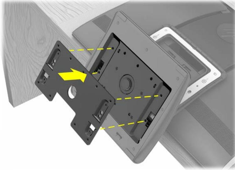
8. Use a Phillips screwdriver to tighten all four screws attaching the VESA adapter plate to the bottom of the computer stand.
