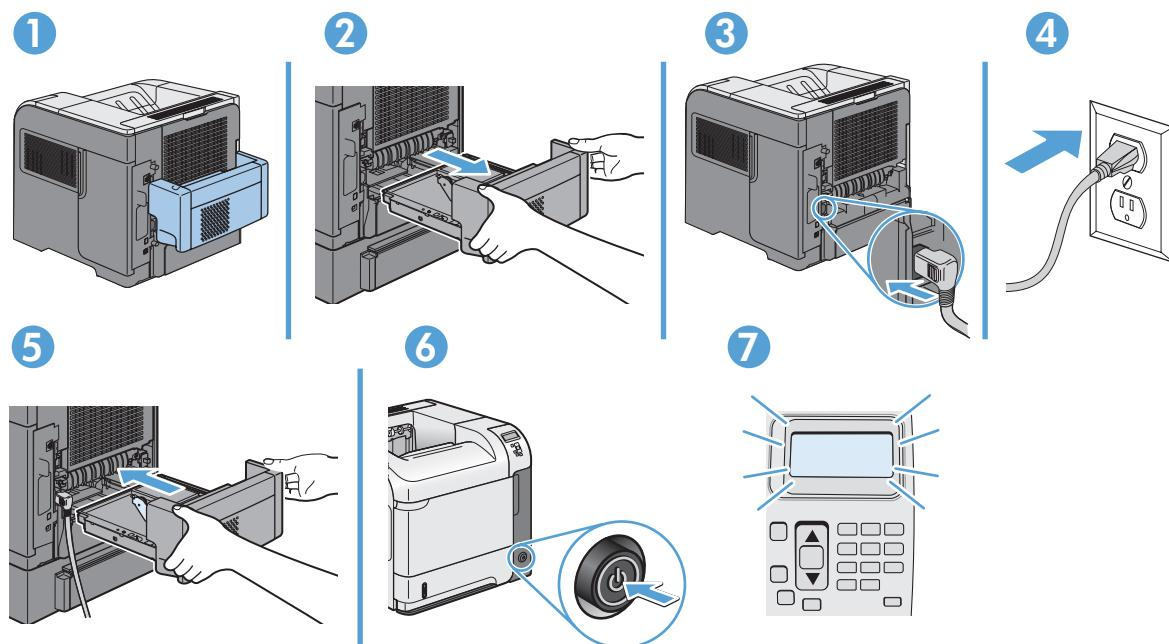
**EN** Connect the power cord between the product and a grounded ac outlet. Turn on the product. On the control panel, set the language and the date/time.
