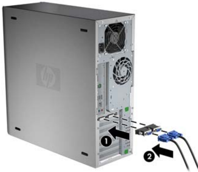
Figure 3-8 Connecting the cables to the workstation
