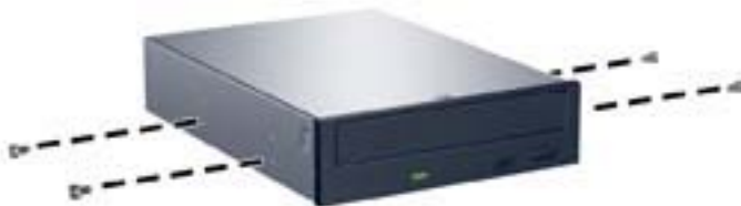
Figure 10-6 Installing Guide Screws in the Optical Drive
