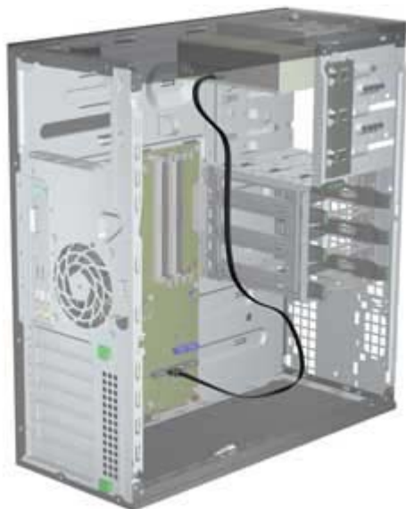
Figure 10-3 Connecting ODD power and data cables
