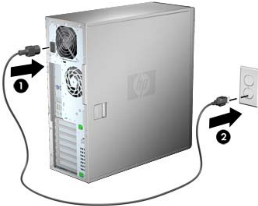
Figure 3-3 Connecting the power cord
