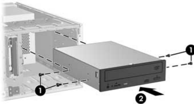
Figure 10-4 Installing the optical drive
