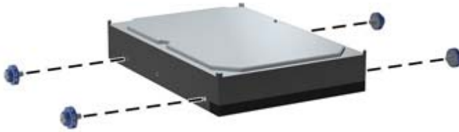
Figure 9-8 Installing the hard drive guide screws
