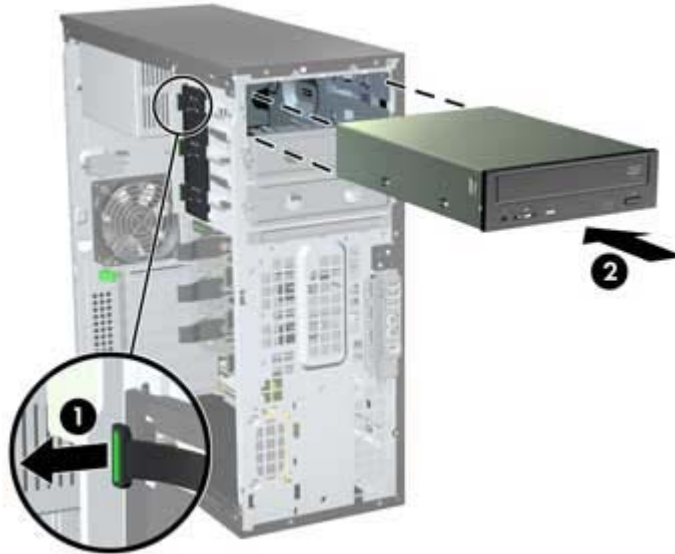
Figure 10-2 Inserting the ODD into the casing
