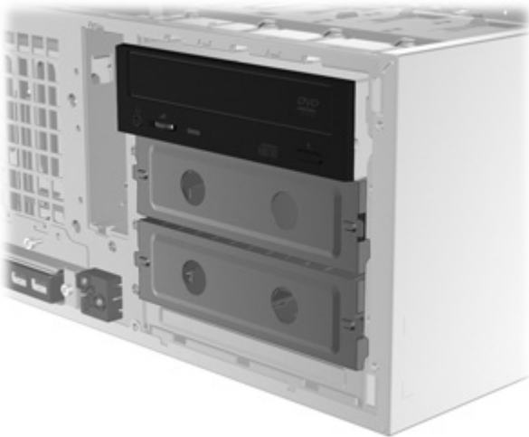
Figure 3-7 Reinstalling the optical drive
