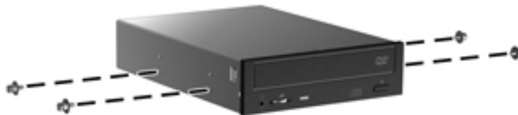
Figure 10-1 Installing the guide screws
