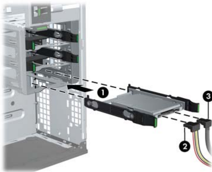
Figure 5-37 Installing the HDD drive
