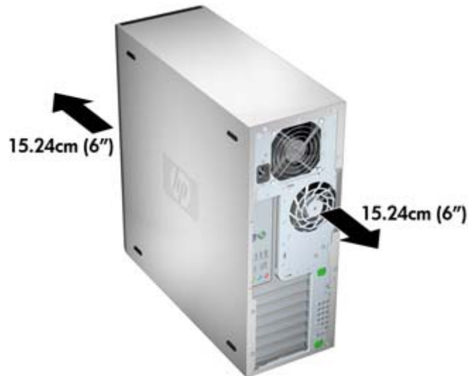
Figure 1-5 Proper workstation ventilation
