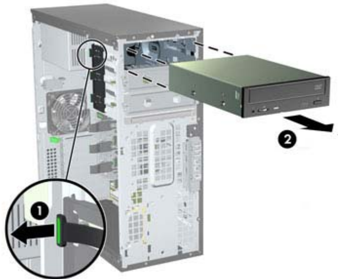
Figure 5-11 Removing the optical disk drive
