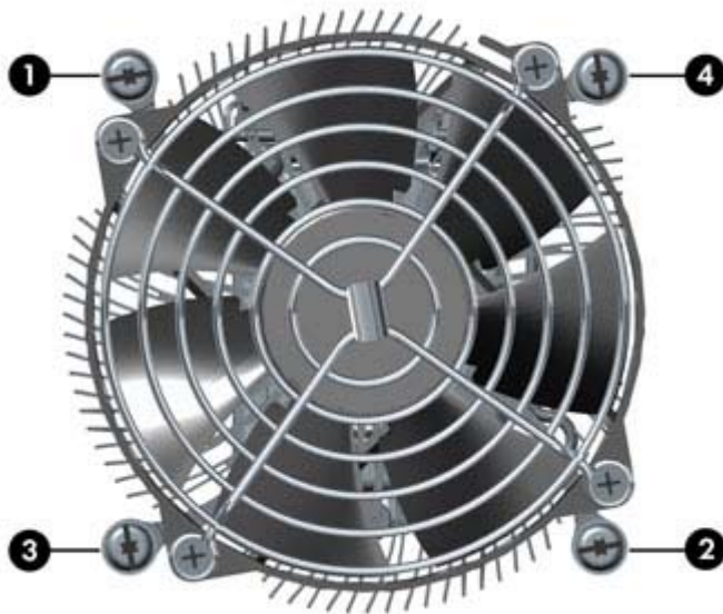
Figure 5-38 Loosening heatsink screws in sequence
