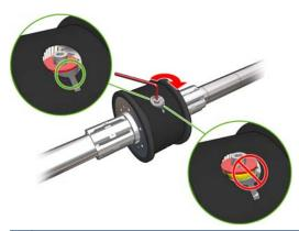
TIP: You should tighten the screw until the washer touches the bolt. If you can still see the yellow spring, tighten the screw further.
