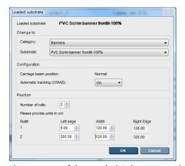
The contents of the Loaded Substrate window are determined automatically when the substrate is loaded and checked. However, if the printer is unable to detect the edges of the substrate (for instance, in the case of a transparent substrate), you will have to measure the distance of the left edge from the printer's side plate, and complete the Left Edge and Width fields yourself.
