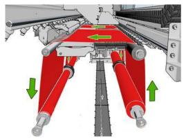
**NOTE:** You can load substrate with the printed face inwards or outwards on the spindle, in which case the spindle will turn in the opposite direction. The printer asks you for the winding direction if it cannot detect it automatically.
