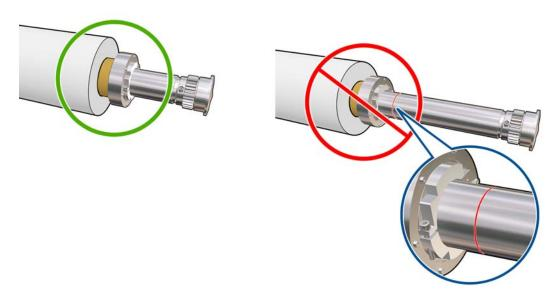
10. Ensure that the roll core fits tightly on the hub.
