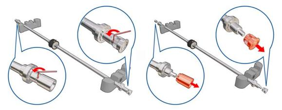
4. Unscrew and remove the inner part of each hub.
