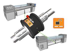
19. Go to the front panel and select the Substrate menu , then **Substrate management**, and press OK. Select **Carriage beam position** > **Move to printing (normal)** to lower the carriage beam into its normal position, close to the substrate. This process takes about 2 minutes to complete.
