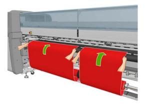
ENWW Load rolls into the printer
