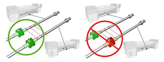
2. When both differential hubs are correctly positioned, use the Allen key to tighten the screws and secure them in place. If a differential hub is loose, the substrate could become skewed during printing.
