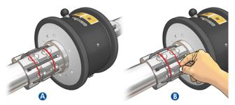
To check to see if the core is slipping on the dual roll, make a mark on the core and the on the differential of the dual roll at the same level, and check if the marks separate as the substrate advances. This type of issue will not trigger an error message, but there will be poor advance accuracy, which will look like banding.
