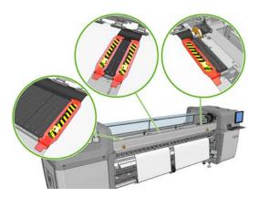
18. Unlock the differentials on the input and output spindles.
