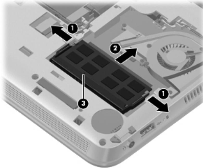
Reverse this procedure to install the memory module.
