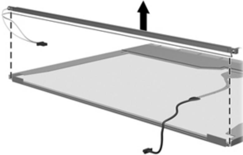
**⚠ WARNING!** The backlight contains mercury. Exercise caution when removing and handling the backlight to avoid damaging this component and causing exposure to the mercury.
