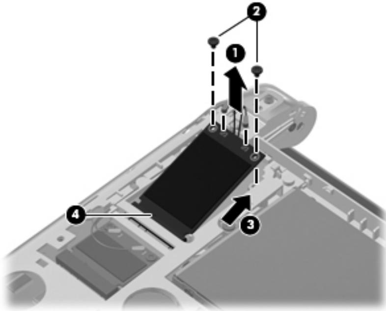
Reverse this procedure to install the WWAN or GPS module.
