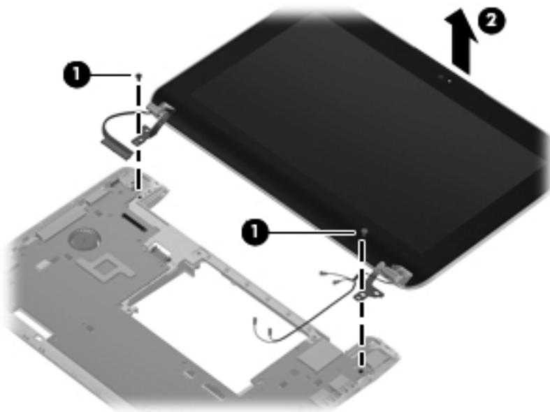
Remove the display assembly hinges:
