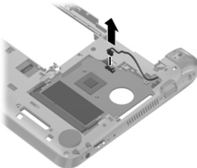
2. Remove the 2 Phillips 2.0×4.0 screws **(1)** that secure the system board to the base enclosure.
