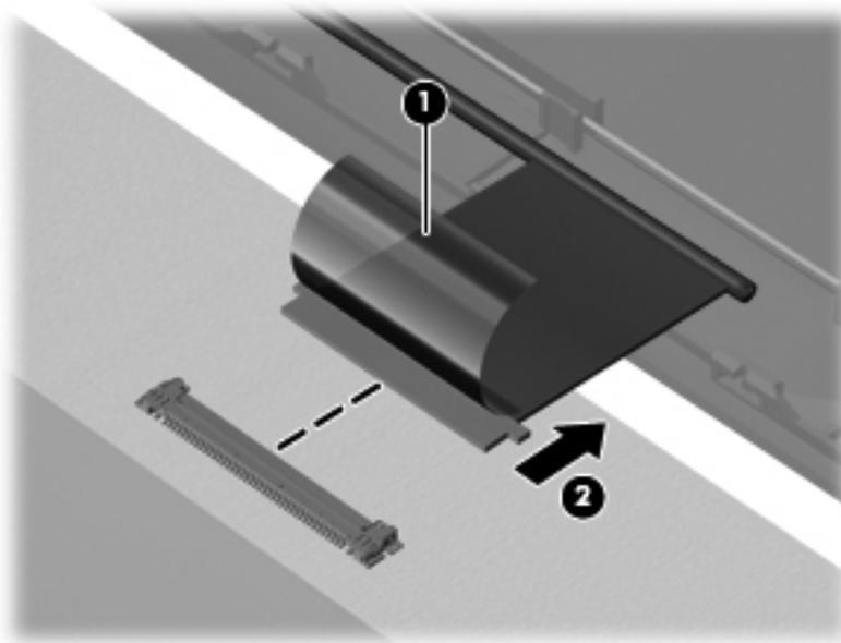
9. Lift the display/webcam cable (1) from its routing path (2) in the display enclosure.
