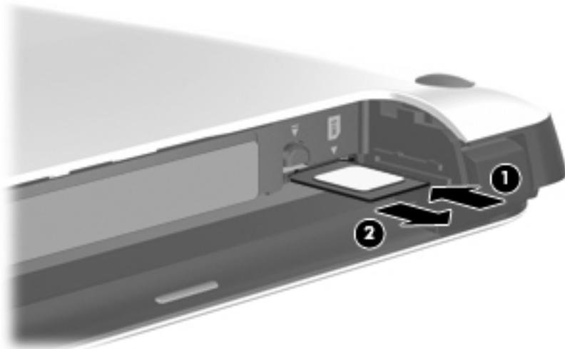
Install the SIM by inserting it into the SIM slot until you hear a click.
