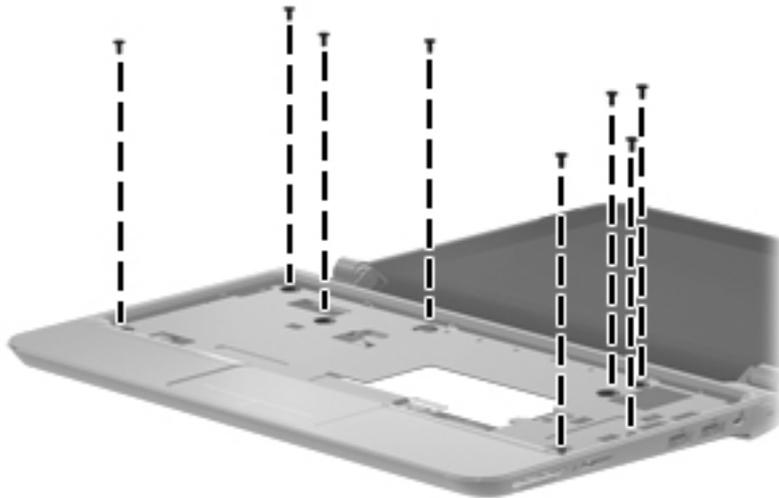
13. Release the top cover by lifting the front edge until it disengages from the base enclosure.
