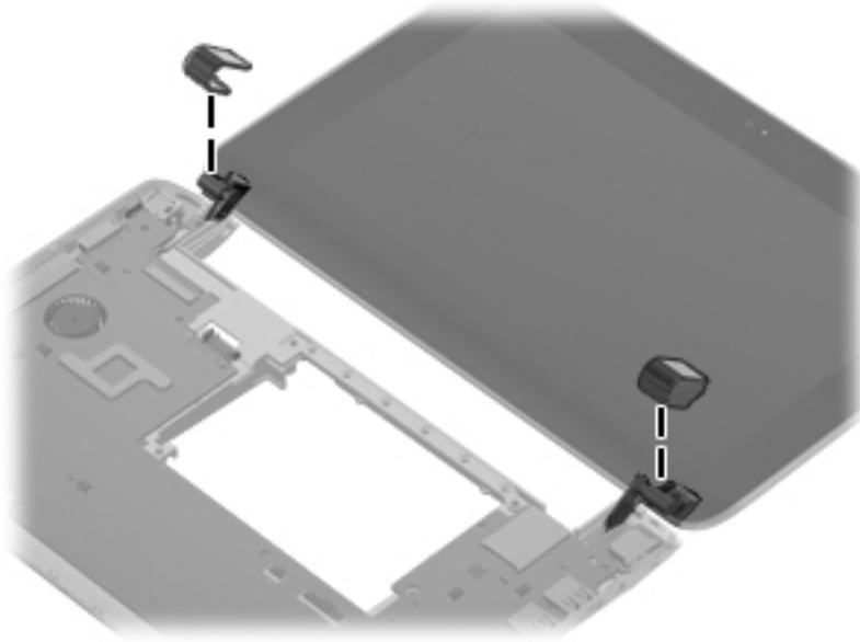
2. Remove the two Phillips 2.0×5.0 screws **(1)** that secure the black plastic covers to the display assembly, and then lift the covers from the display **(2)**.
