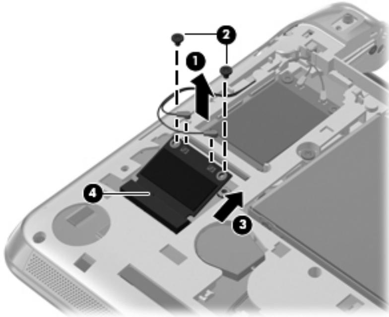
Reverse this procedure to install the WLAN module.
