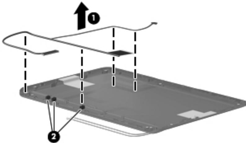
10. If you need to remove the antenna cables, lift the cables (1) from the routing path (2) in the display enclosure. The antenna cables are available using spare part number 631698-001 for use in computers that do not use LTE WWAN modules and 638146-001 for use in computers that use LTE WWAN modules.
