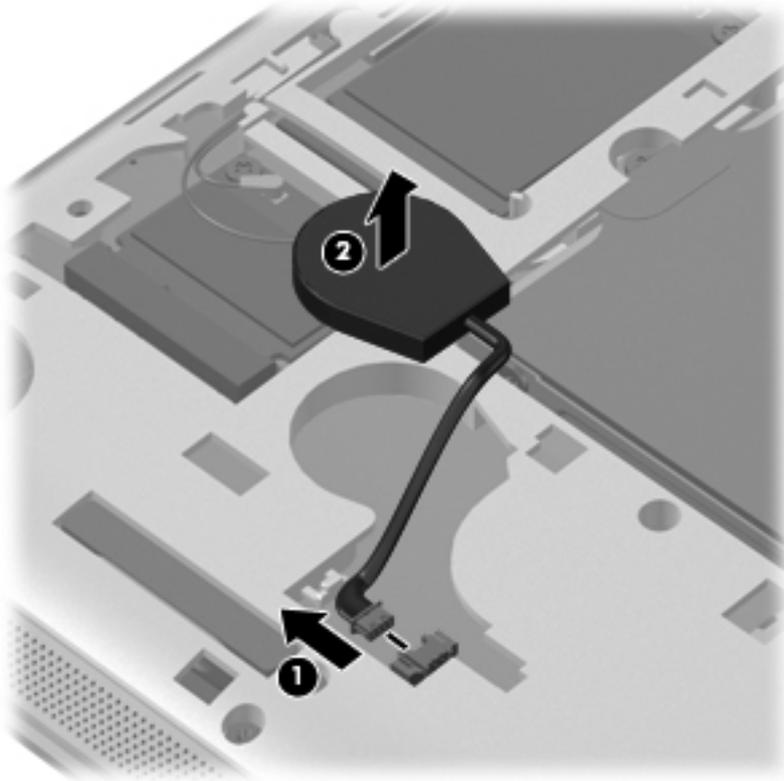
Reverse this procedure to install the RTC battery. When installing the RTC battery, be sure the plus sign (+) faces up.
