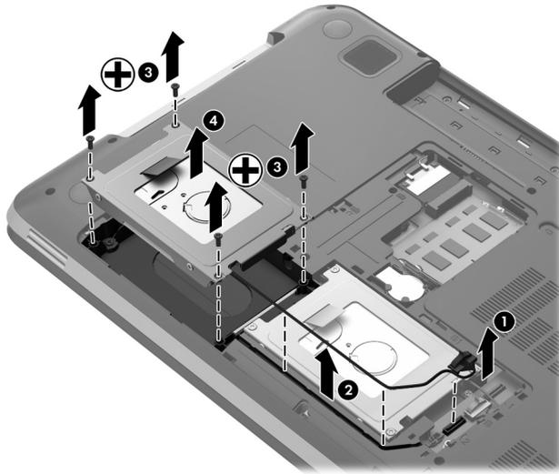
8. If it is necessary to replace the hard drive bracket or hard drive connector cable:
