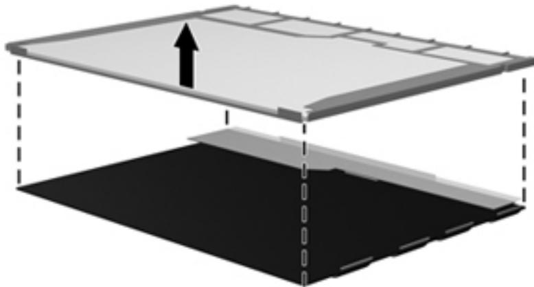
**24.** Recycle the LCD panel and backlight.
