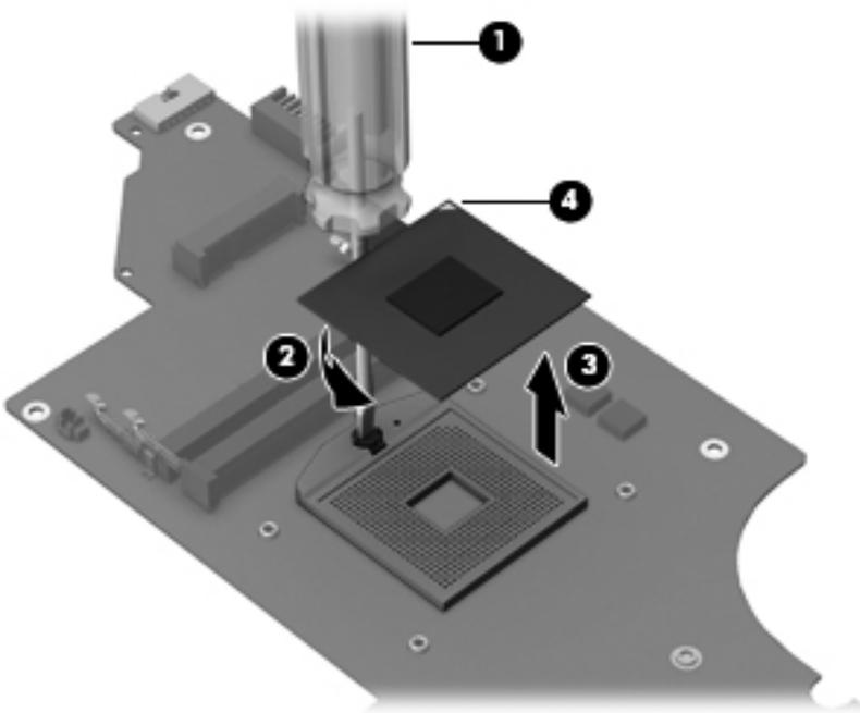
Reverse this procedure to install the processor.
