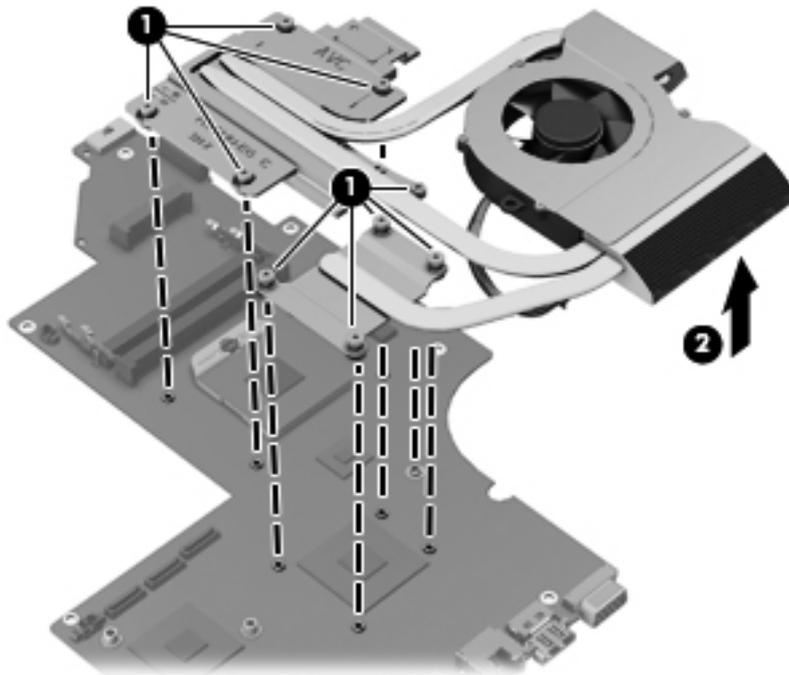
**NOTE:** The thermal material must be thoroughly cleaned from the surfaces of the heat sink and the system board components each time the fan/heat sink assembly is removed. Replacement thermal material is included with the fan/heat sink assembly, processor, and system board spare part kits.
