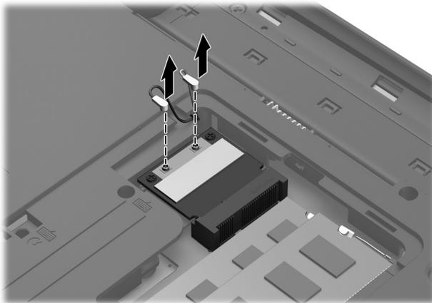
2. Remove the two Phillips PM2.0x4.0 screws that secure the WLAN module to the system board. (The WLAN module tilts up.)
