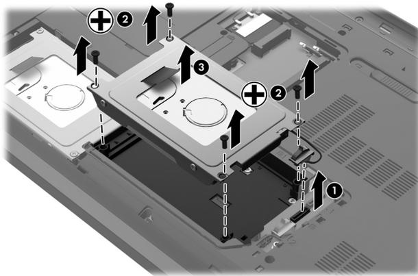
4. Disconnect the hard drive cable **(1)** from the system board.
