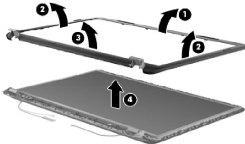
**5.** If it is necessary to replace the display panel:
