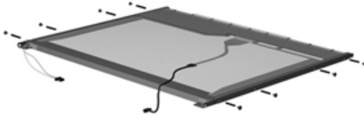
**11.** Remove the screws **(1)** that secure the backlight cover to the display panel.
