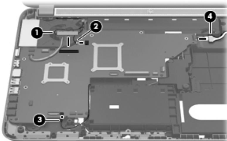
7. Remove the five Phillips PM2.5x5.0 screws that secure the system board to the base enclosure.
