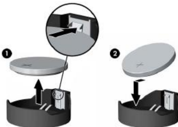
Figure 5-40 Removing the battery from a type 2 holder
