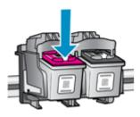
**4.** Hold the ink cartridge by its sides with the bottom pointing up and locate the electrical contacts on the ink cartridge. The electrical contacts are four small rectangles of copper or gold-colored metal on the bottom of the ink cartridge.
