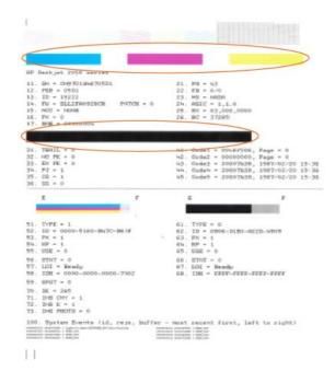
6. Clean the print cartridges automatically, if the diagnostic page shows steaks or missing portions of the color and black boxes.
