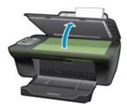
Load original print side down on right front corner of glass.
