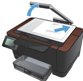
**EN** **Test the copy function.** Raise the camera arm to the fully open position. Load a printed page onto the capture stage, face-up. Align the page with the raised guides at the left and rear edges. On the control panel, touch **Copy** and then touch **Black** to start copying.
