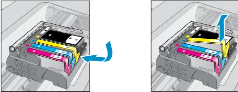
4. Hold the ink cartridge by its sides with the bottom pointing up and locate the electrical contacts on the ink cartridge. The electrical contacts are four small rectangles of copper or gold-colored metal on the bottom of the ink cartridge.
