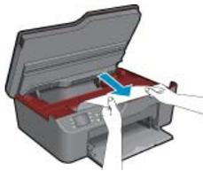
2. If the paper jam is located towards the back of the printer, open the cleanout door to access.
