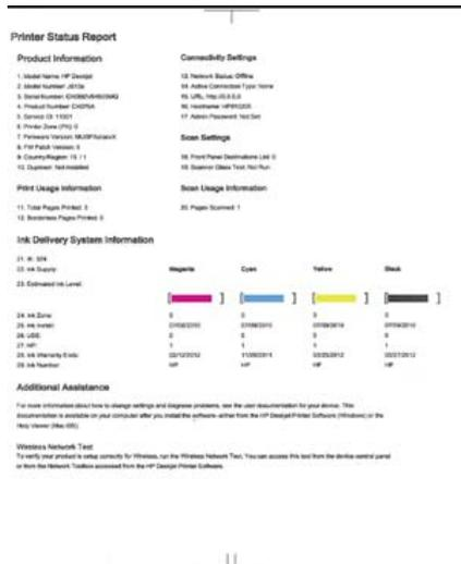
6. Clean the print cartridges automatically, if the diagnostic page shows streaks or missing portions of the color and black boxes.
