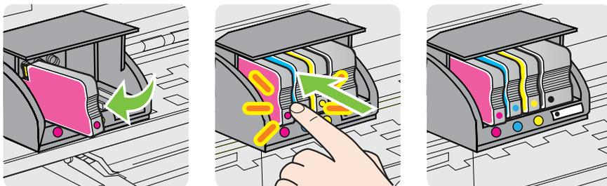
Make sure that you insert the ink cartridge into the slot that has the same colored letter as the color you are installing.
