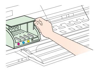
**4.** Remove the printhead by lifting it up and then pulling it out of the printer.
