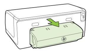
Reinsert the duplexer into the printer.
