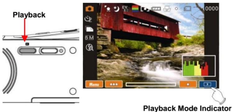
2. Press 4-Way Direction Button up/down, or left/right to view the stored files. Press Menu (
