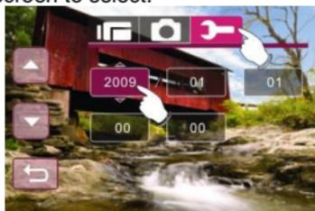
2. Press the 4-Way Direction Button left/right to highlight each column. Then press up/down or touch the screen to select the column.
