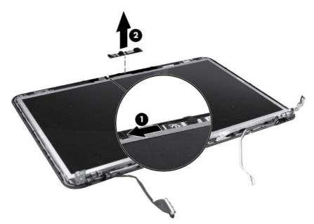
Reverse this procedure to install the webcam module.
