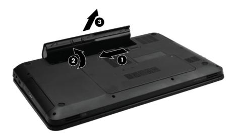
To insert the battery, insert the rear edge of the battery into the battery bay and pivot the front edge downward until the battery is seated. The battery release latch automatically locks the battery into place.
