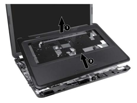
NOTE: The TouchPad is glued to the top cover and is included with the top cover spare part.
