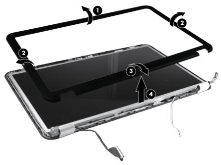
Reverse this procedure to install the display bezel.
