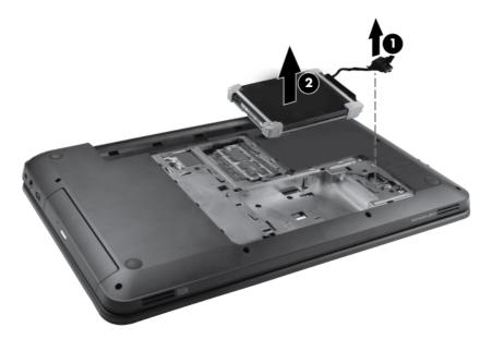
Disconnect the hard drive adapter (1). Then remove the hard drive bumpers (2), and the cover (3).
