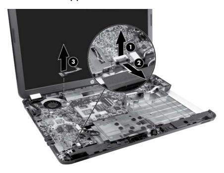
Reverse this procedure to install the TouchPad LED board.
