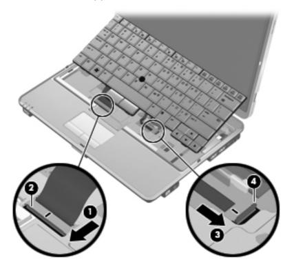
**15.** Align the tabs on the keyboard with the notches on the computer **(1)** and replace the keyboard **(2)**.
