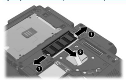
To protect a memory module after removal, place it in an electrostatic-safe container.
