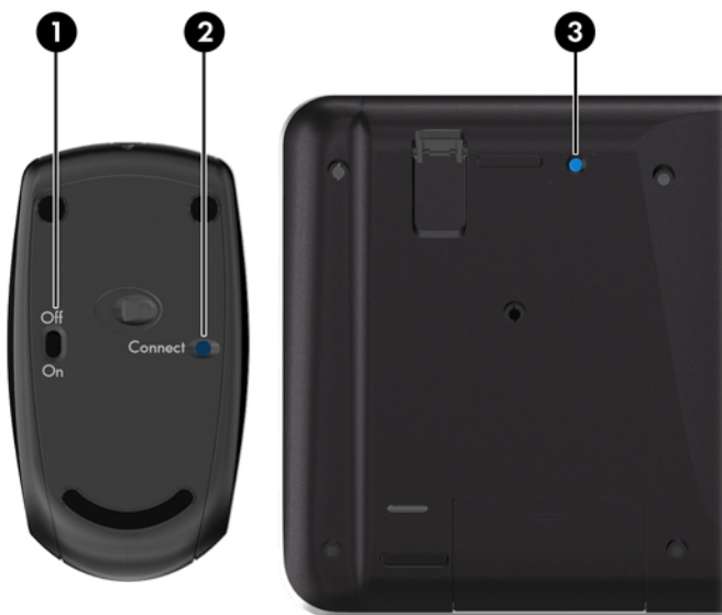
Figure 2-24 Synchronizing the Wireless Keyboard and Mouse
