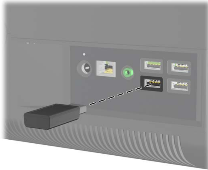
Gambar 2-23 Memasang Receiver Nirkabel
