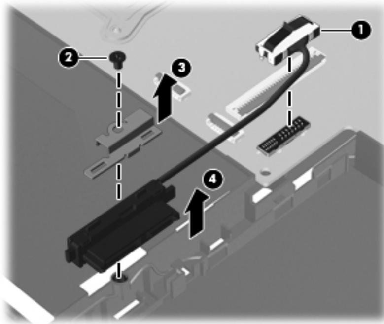
Reverse this procedure to install the optical drive connector cable.
