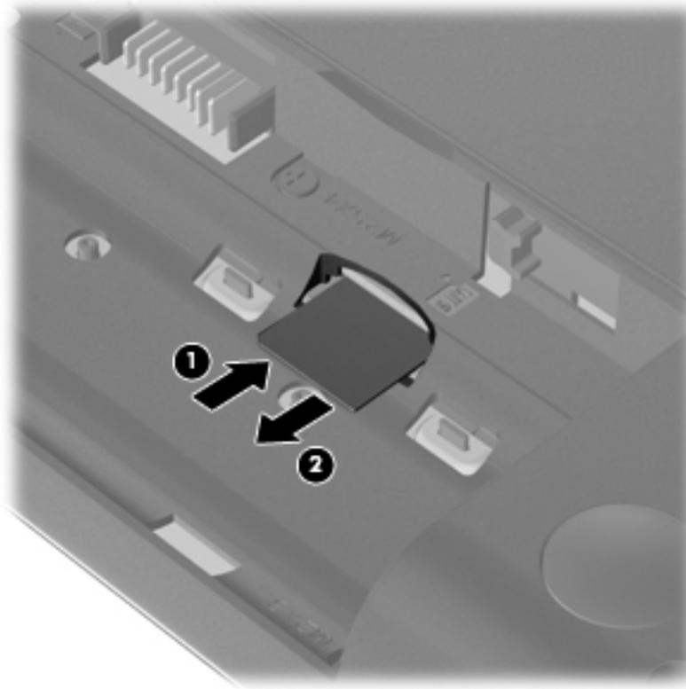
Insert the SIM into the SIM slot, and gently push the SIM into the slot until it is firmly seated.
