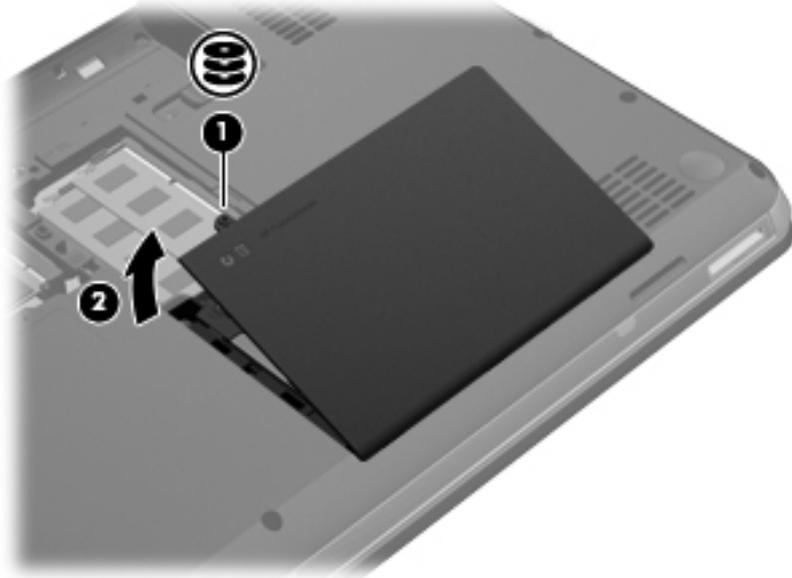
3. Remove the hard drive compartment cover. The hard drive compartment cover is available in the Plastics Kit, spare part number 650478-001.
