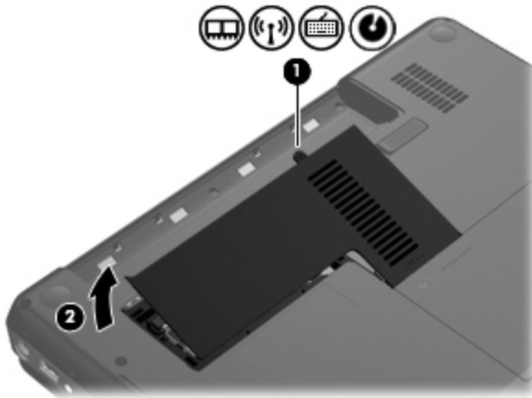
3. Remove the memory module/wireless module compartment cover. The memory module/wireless module compartment cover is available in the Plastics Kit, spare part number 650478-001.
