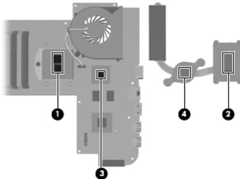
The following illustration shows the replacement thermal material locations on a computer model equipped with an AMD processor and a graphics subsystem with UMA memory.
