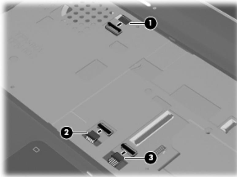
8. Lift the rear edge of the top cover **(1)** until the left and right sides disengage from the base enclosure.
