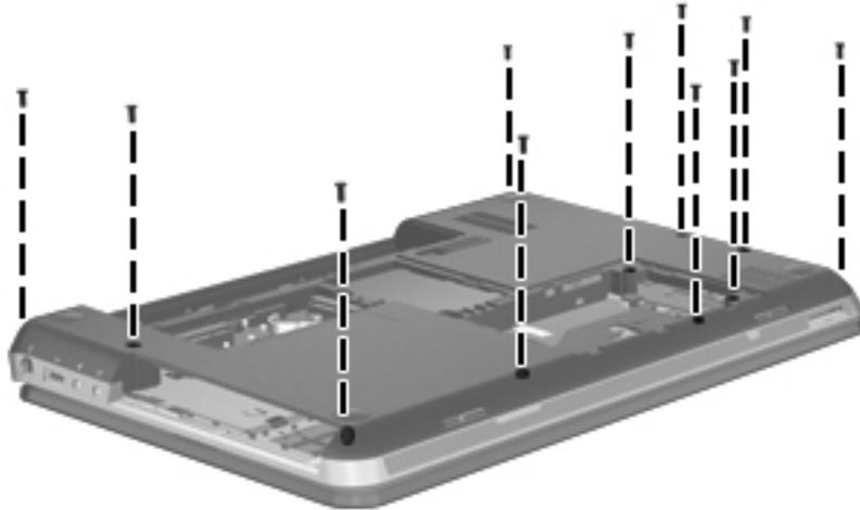
4. Remove the following screws that secure the top cover to the computer:
