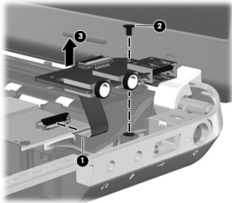
Reverse this procedure to install the audio/USB board.
