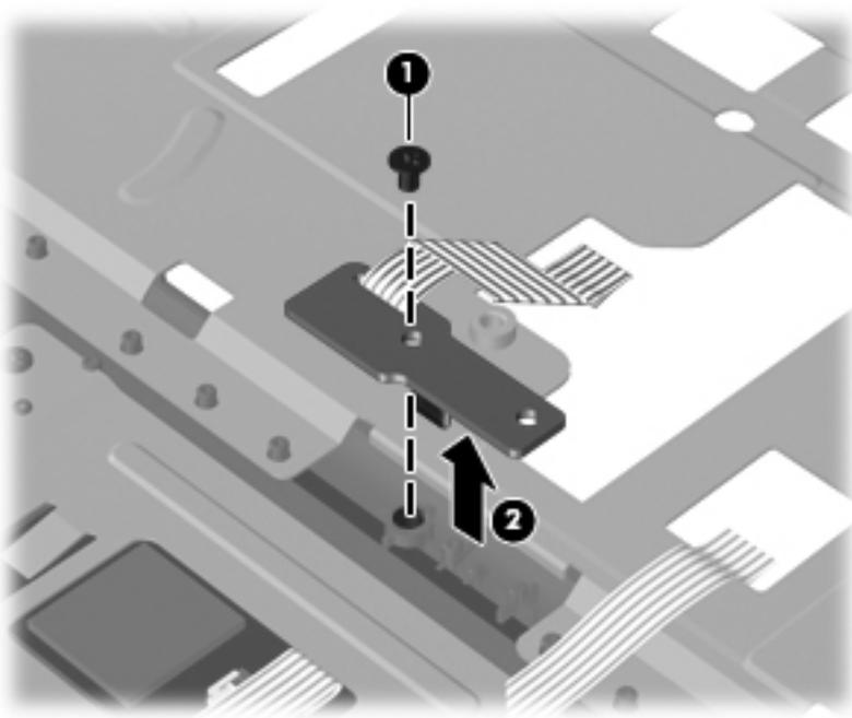
Reverse this procedure to install the TouchPad LED board and cable.
