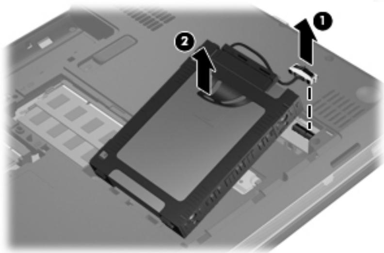
6. If it is necessary to replace the hard drive connector cable (1), the hard drive screws (2), or the hard drive bracket (3), remove and replace the components.
