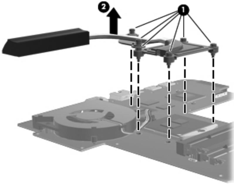
The following illustration shows the heat sink removal process on a computer model equipped with an Intel processor and a graphics subsystem with discrete memory.
