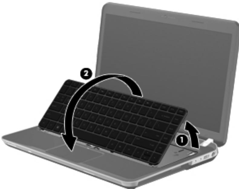
7. Release the zero insertion force (ZIF) connector **(1)** to which the keyboard cable is attached, and then disconnect the keyboard cable **(2)** from the system board.
