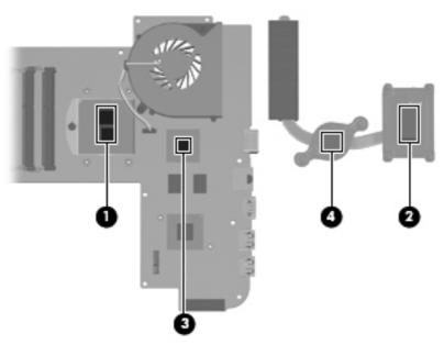
The following illustration shows the replacement thermal material locations on a computer model equipped with an AMD processor and a graphics subsystem with UMA memory.
