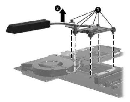
The following illustration shows the heat sink removal process on a computer model equipped with an AMD processor and a graphics subsystem with UMA memory.
