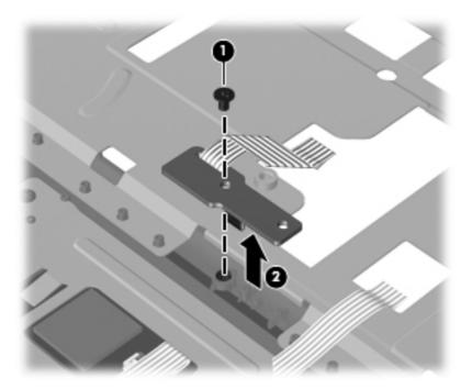
Reverse this procedure to install the TouchPad LED board and cable.
