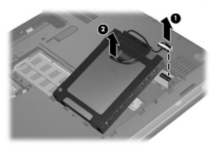
**6.** If it is necessary to replace the hard drive connector cable **(1)**, the hard drive screws **(2)**, or the hard drive bracket **(3)**, remove and replace the components.
