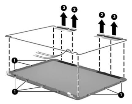
**c.** Remove the wireless antenna cables and transceivers. The WLAN antenna are available using spare part number 650444-001. The WWAN antenna are available using spare part number 650445-001.
