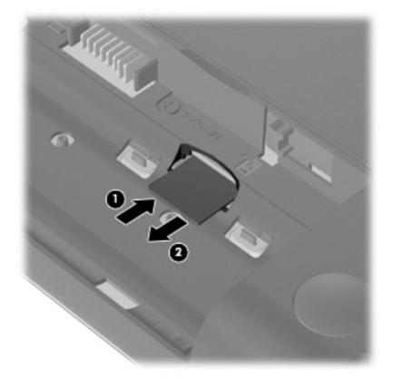
Insert the SIM into the SIM slot, and gently push the SIM into the slot until it is firmly seated.
