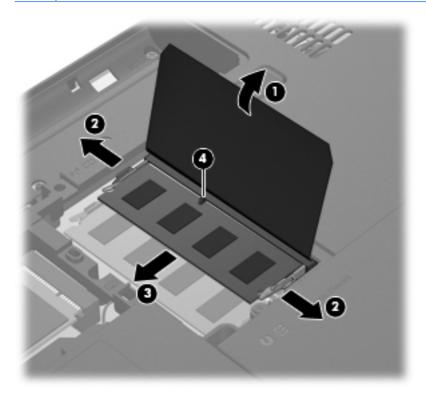
Reverse this procedure to install a memory module.
