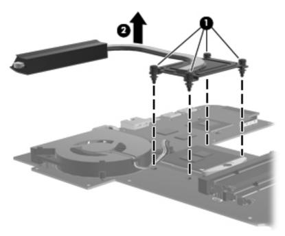
NOTE: The thermal material must be thoroughly cleaned from the surfaces of the heat sink and the system board components each time the heat sink is removed. Replacement thermal material is included with the base enclosure, heat sink, processor, and system board spare part kits.
