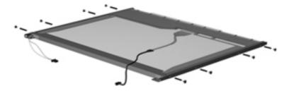
Use a sharp-edged tool to cut the tape (1) that secures the sides of the display panel to the display panel frame. 10. Remove the display panel frame (2) from the display panel.
