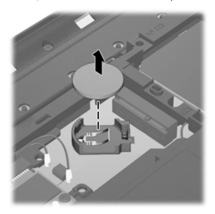
Reverse this procedure to install the RTC battery. When installing the RTC battery, make sure the "+" sign faces up.
