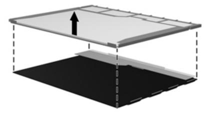
**24.** Recycle the LCD panel and backlight.
