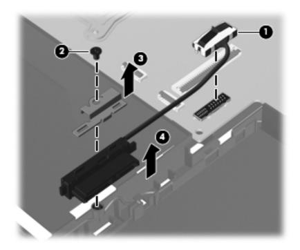
Reverse this procedure to install the optical drive connector cable.
