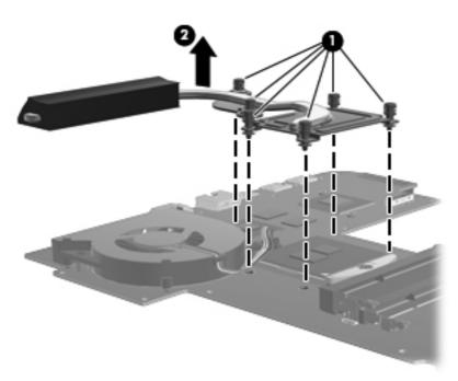
The following illustration shows the heat sink removal process on a computer model equipped with an Intel processor and a graphics subsystem with UMA memory.
