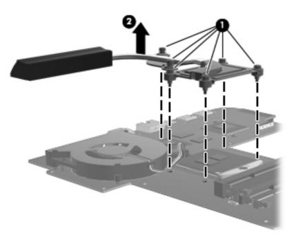
The following illustration shows the heat sink removal process on a computer model equipped with an Intel processor and a graphics subsystem with discrete memory.
