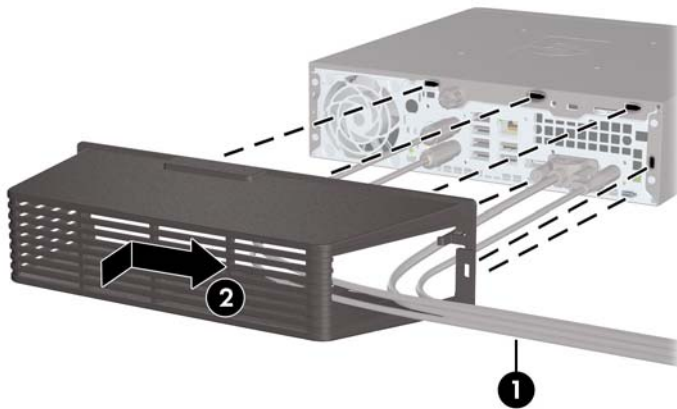
Figure 2-22 Installing a Port Cover
