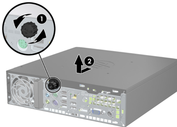
Figure 2-2 Removing the Computer Access Panel
