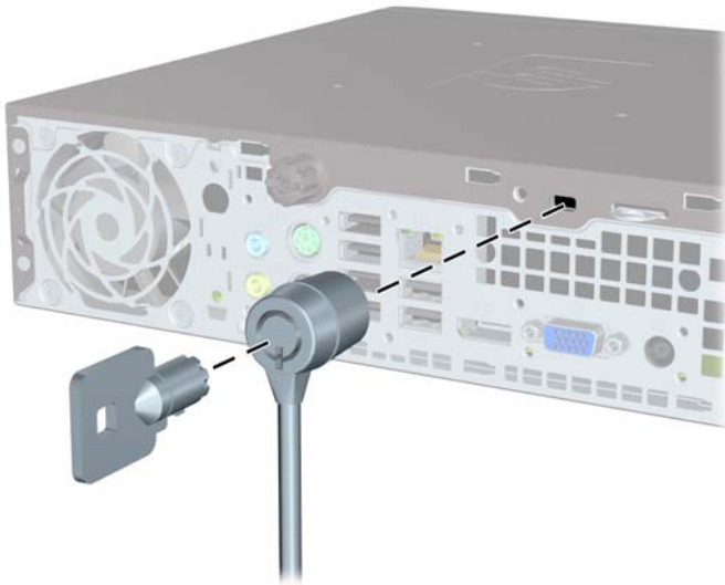
Figure 2-25 Installing a Cable with a Port Cover Installed
