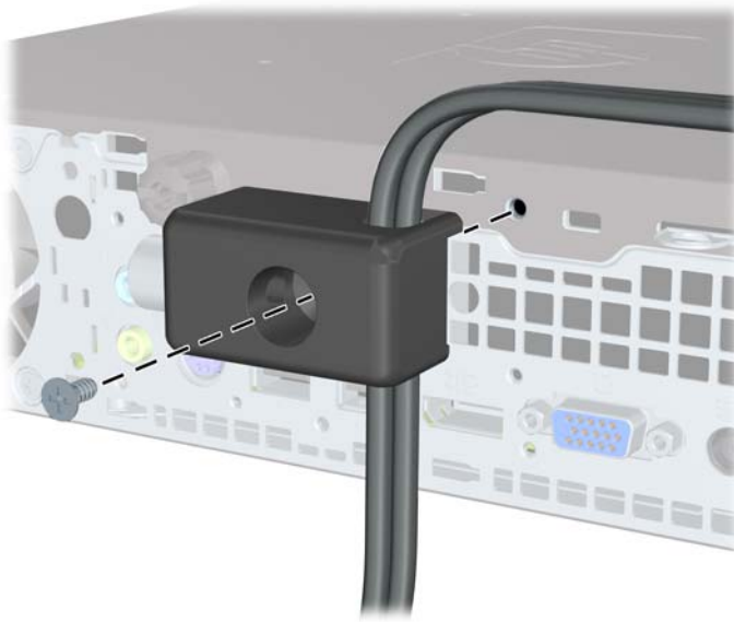
Figure 2-32 Attaching the Lock to the Chassis
