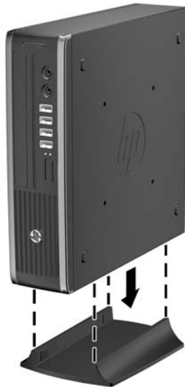
Figure 2-7 Placing the Computer on the Stand
