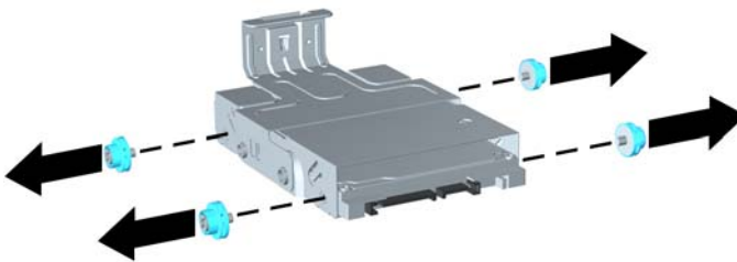
Figure 2-17 Removing the Guide Screws
