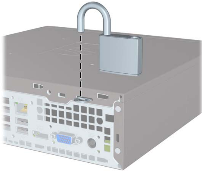
Figure 2-26 Installing a Padlock
