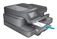
Slide stack of envelopes forward until it stops. Slide paper-width guide inward against stack of envelopes until it stops.
