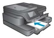
Slide stack of paper forward until it stops. Slide paper-width guide inward until it stops at edge of paper.
