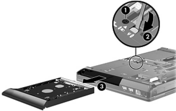
6. Remove the assembly from the base enclosure.
