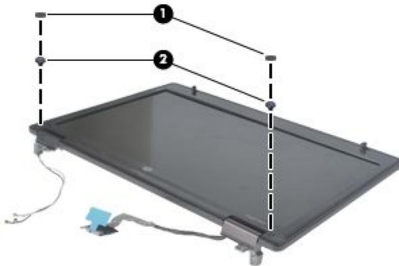
9. Flex the top of the bezel, the inside edges of the left and right sides **(1)**, and then the top and bottom **(2)** of the bezel until it disengages from the display enclosure.
