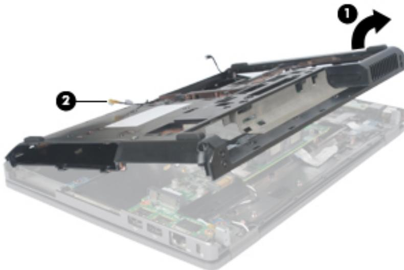
**⚠ CAUTION:** When installing the base enclosure, be sure that the wireless antenna cables routed out of the display assembly are routed and arranged properly.
