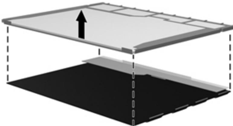
24. Recycle the LCD panel and backlight.
