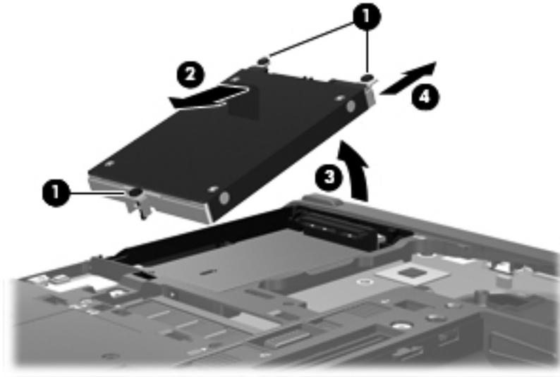
5. If it is necessary to replace the hard drive bracket, remove the four Phillips PM3.0×5.0 hard drive bracket screws (1) from each side of the hard drive.
