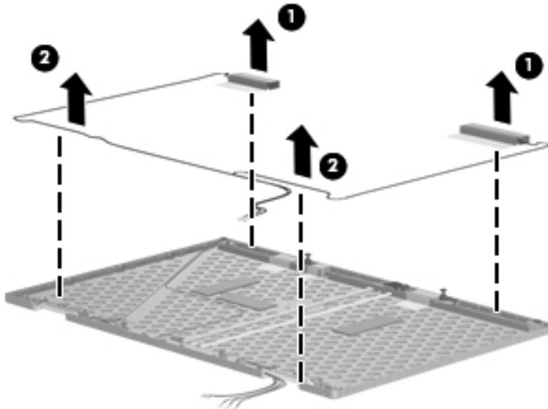
19. If it is necessary to remove the WLAN antenna transceivers (1) and cables, remove them from the display enclosure back cover by lifting them (2) from the clips in the display enclosure back cover.
