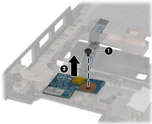
Reverse this procedure to install the Power button board assembly.
