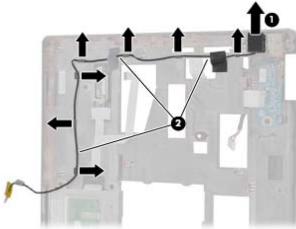
4. Remove the RJ-11 connector cable from the top cover.
