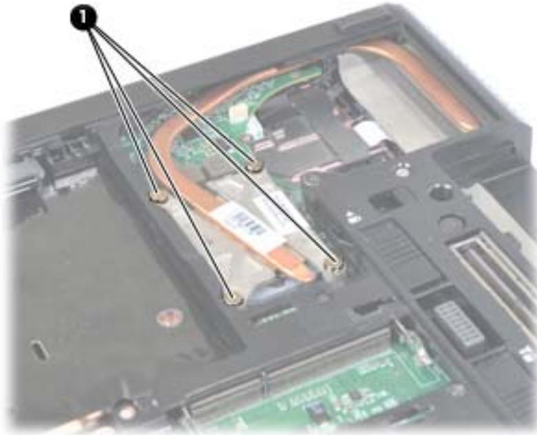
3. Lift the right side of the heat sink (1) to disengage it from the system board.
